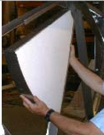
Figure 14. Slide segment on spoke until contacts stop in hub plate.
