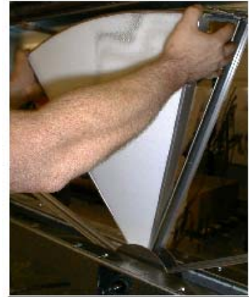
Figure 11. Insert nose of segment between hub plates to install
