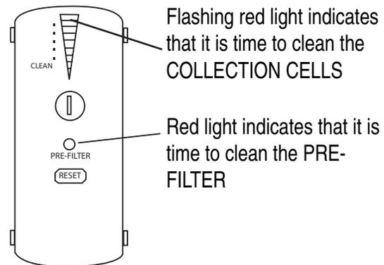
Flashing red light indicates that it is time to clean the COLLECTION CELLS
