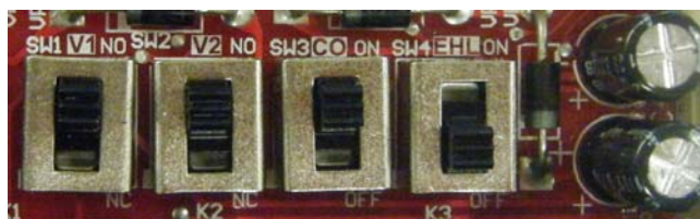
Figure 88. CSTI adapter board: board-mounted switches
