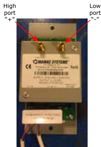
Figure 143. Fan inlet airflow measuring system
