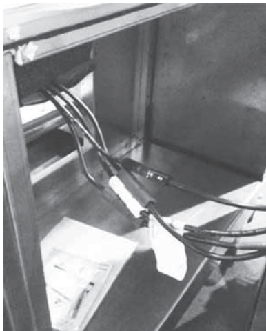
Figure 29. Horizontal section-to-section high voltage quick connects
