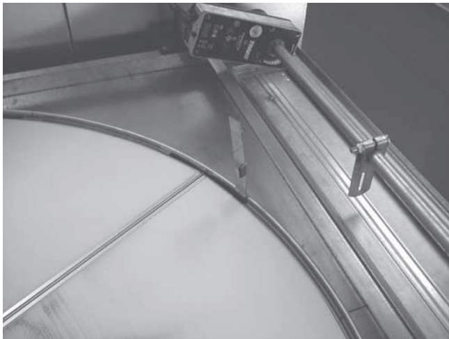
Figure 145. Confirm proper belt tracking on the wheel rim
