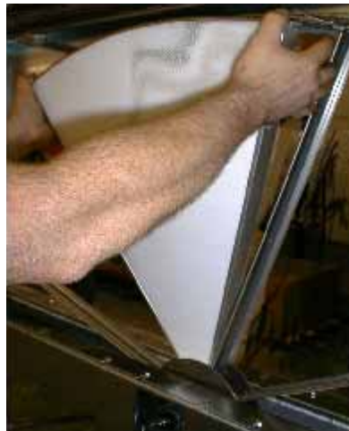
Figure 144. Insert nose of segment between hub plates to install
