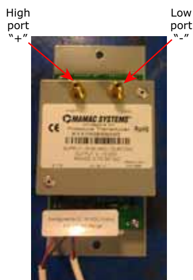
Figure 139. Fan inlet airflow measuring system
