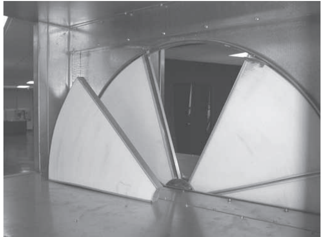
Figure 144. Insert nose of segment between hub plates to install
