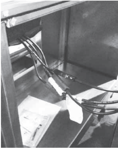
Figure 29. Horizontal section-to-section high voltage quick connects
