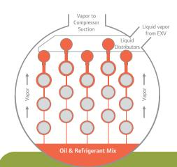
Our patented evaporator design gives the Trane RTWD higher efficiencies using less refrigerant charge, both of which contribute to LEED certification. over the first row of tubes. It then flows around them, precisely at the points where heat transfer occurs, to more efficiently cool the fluid (blue) inside.
