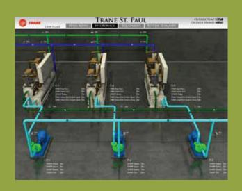
Our most sophisticated control system, Tracer Summit, brings your entire building, or even an entire enterprise, together on one screen with extensive standard and custom reporting. It extends Trane Chiller Plant Control to include optimization of the air handling side of your system, which often uses as much or more energy as the refrigeration side of the system. Focusing on overall system efficiency translates to more reliable system performance and greater energy savings.
