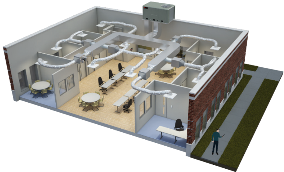
Figure 14. Packaged rooftop example
