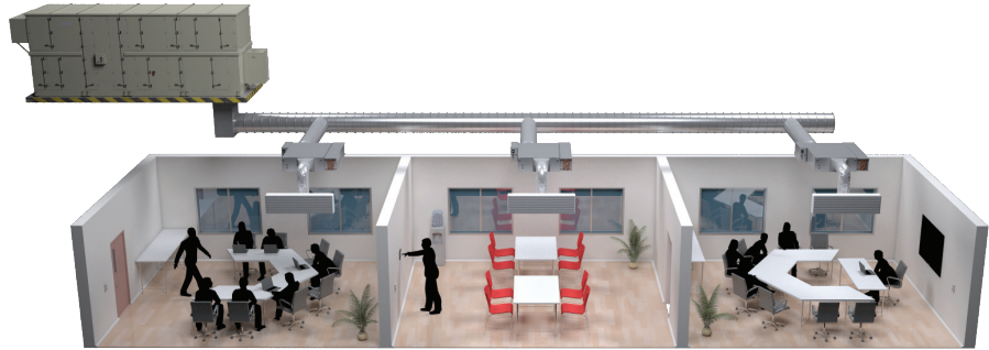
Figure 15. Air handling system example
