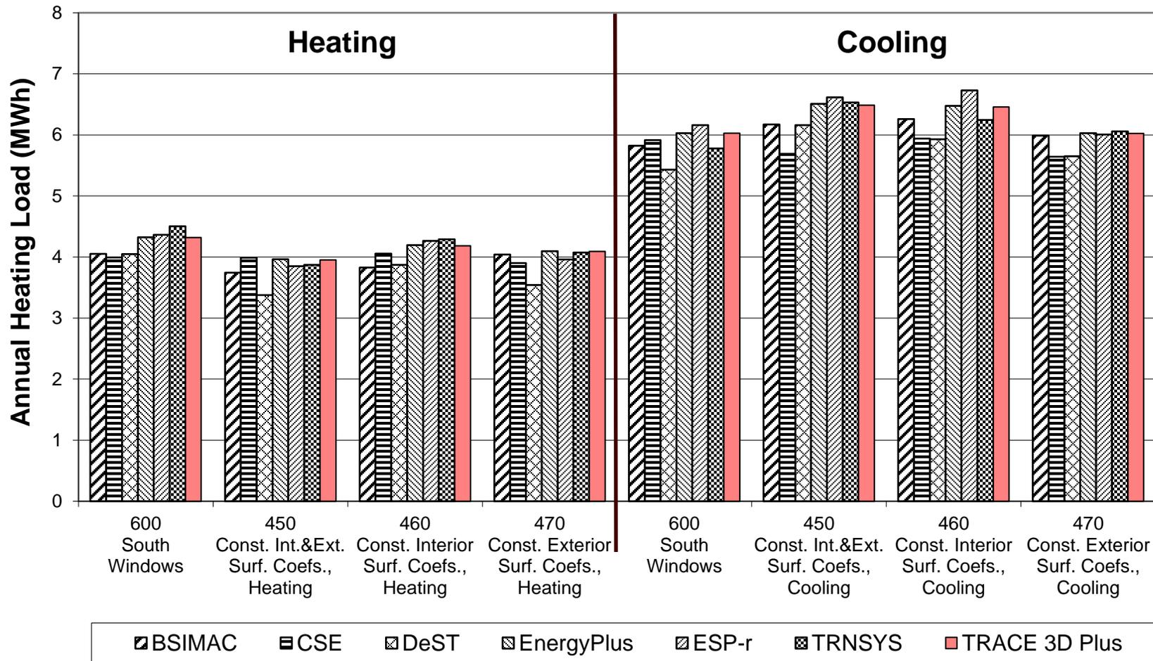
**Figure B8-57. In-Depth: Surface Heat Transfer
