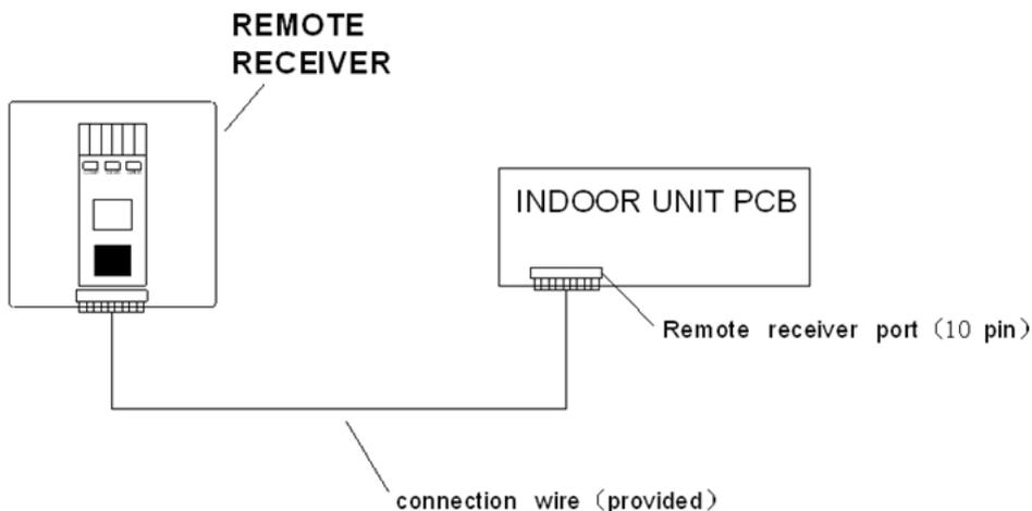
To find the remote receiver port on indoor unit PCB (please refer to the indoor unit wiring diagram)
