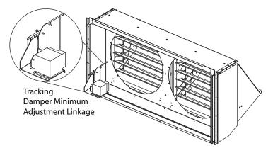
Figure 48. (Horizontal) Tracking Exhaust Damper Adjustment
