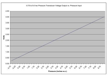
Figure 41. Transducer Voltage Output vs. Pressure Input for Supply, Return and Building Pressure
