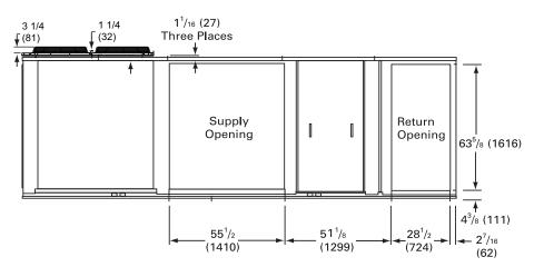
Figure 5. Duct openings, 60 Hz 271/2-35, 50 Hz 23-29 Tons (YC High Heat)
