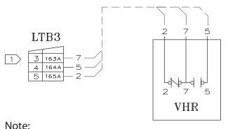
Heat mode/unoccupied mode relay output to VAV
