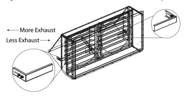
Figure 49. (Downflow) Standard Exhaust Maximum Damper Position
