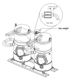
Figure 53. Line Weight Locations-50 Ton
