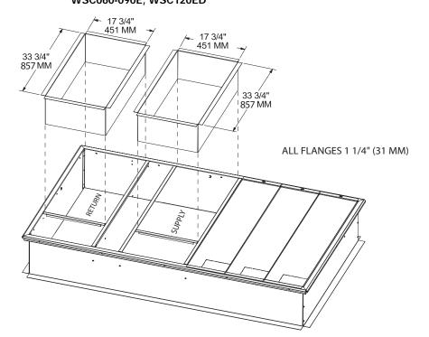
Figure 14. Curb dimensional data — T/YSC072-102E, T/YSC120F, T/YHC047-072E, T/YHC092F, WSC060-090E, WSC120ED
