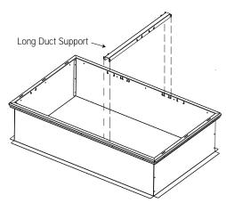
4. Insert the other two long duct supports as shown. See Figure 2, p. 7. Verify the 4.88" and 16.75" dimensions between long duct supports.
