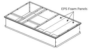
8. Install three pieces of foam insulation and gasket. See Figure 12.
