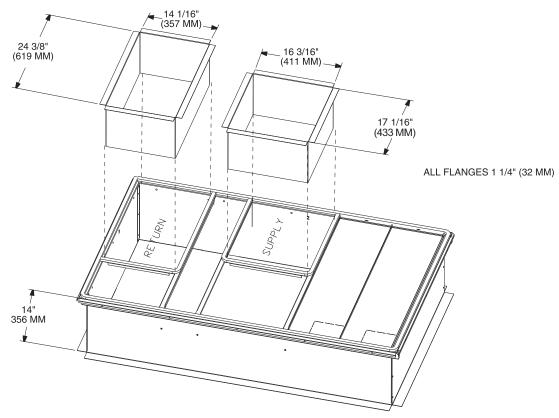
Figure 7. Curb dimensional data T/YSC036-060E, T/YHC036E, T/YHC037E, WSC036-060ED
