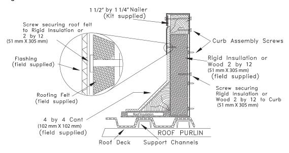
2 by 2 Nailer Strip (Kit supplied) Screw securing roof felt to Rigid Insulation or 2 by 12 > Curb Assembly Screws (51 mm X 305 mm) Rigid Insullation or Flashing Wood 2 by 12 (51 mm X 305mm) (field supplied) (field supplied) Screw securing Rigid Insulation or Wood 2 by 12 to Curb Roofing Felt (field supplied) Wood Nailers (field supplied) 4 by 4 Cant (102 mm X 102 mm) (field supplied) ROOF **PURLIN** Roof Deck
