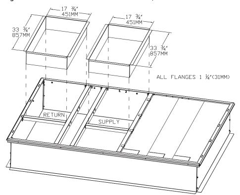
Figure 21. Curb dimensional data — T/YHC092-120E,WSC120E
