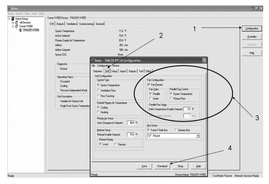
Figure 24. VV550 configuration: temperature setpoints
