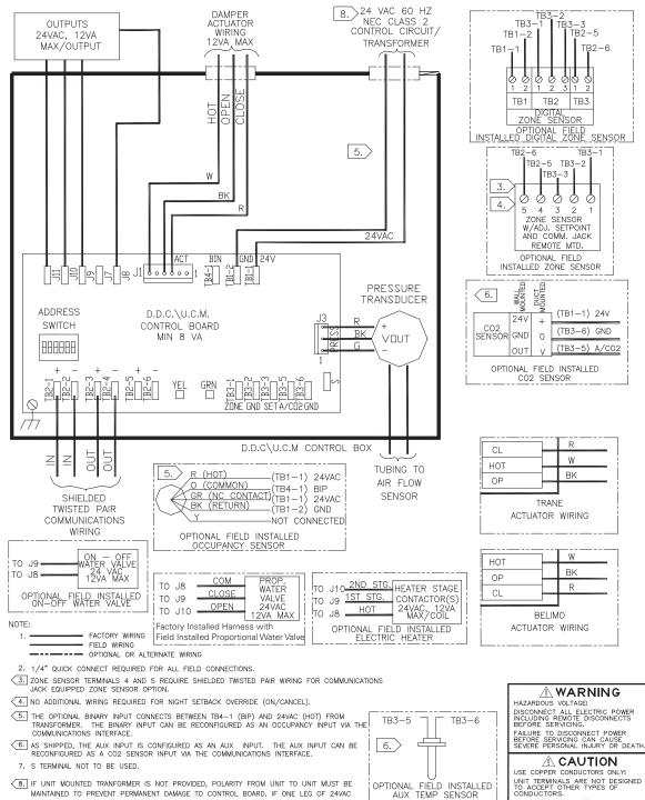
MAINTAINED TO PREVENT PERMANENT DAMAGE TO CONTROL BOARD. IF ONE LEG OF 24VAC SUPPLY IS GROUNDED, THEN GROUND LEG MUST BE CONNECTED TO TB1-2.
