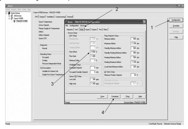
To Set the Measured Value for Airflow
