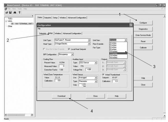
Figure 17. UCM 4.2 configuration: setup inlet size
