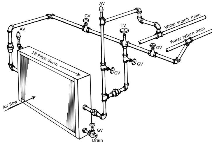
Figure 57. Typical piping for stacked water coils
