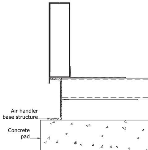
**Figure 20. Flat base to steel dunnage**
