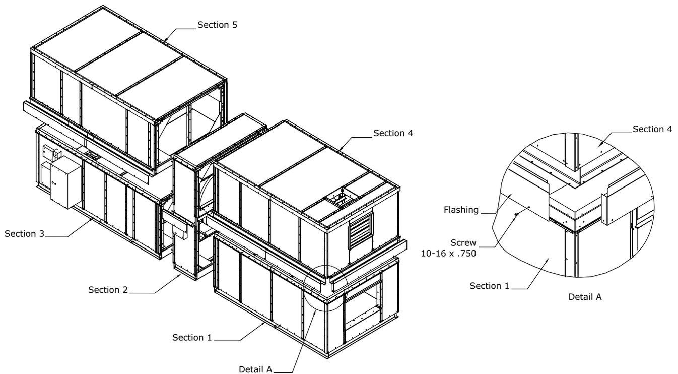
2. Prior to upper unit placement, install 0.188-in. x 2-in. gasketing on entire length of engagement plate and/or lower unit perimeter as needed. Engagement plates are used when the upper and lower unit dimensions are not matched. Refer to "[TCC Stacking Procedure](#)" on page 40.
