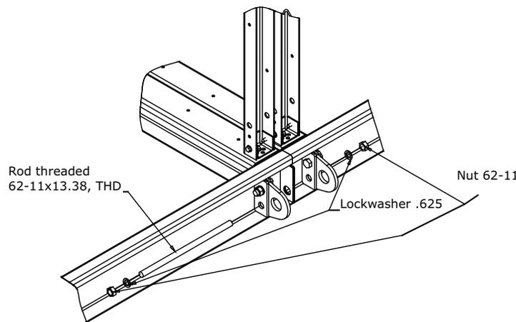
Figure 26. Insert threaded rods
