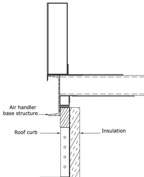
The TCP unit exterior base channel is constructed to overhang the roof curb. Unit support is provided by a square tube channel located inside of exterior base channel. See [Figure 4](#). The standard curb should be designed to properly support the unit's weight without bow and sized to fit within the perimeter base channel.
