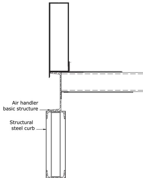
Figure 6. I-beam dunnage mount
