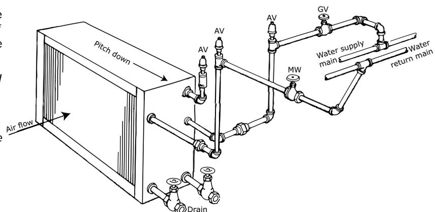
Figure 56. Typical piping for type W or WA 1-row water coil
