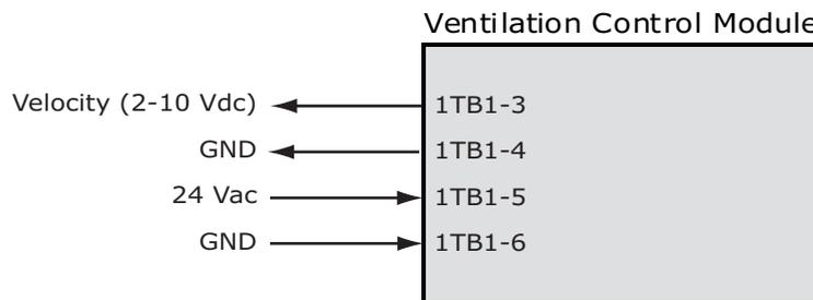
Traq dampers are low-leak dampers that modulate and measure airflow. Each Traq damper section is supplied with a factory-mounted ventilation control module (VCM) on the interior of the mixing box. The VCM has an input terminal for power and an output terminal for air velocity (see [Figure 76](#)). A direct-digital controller controls the factory-mounted and wired actuators.
