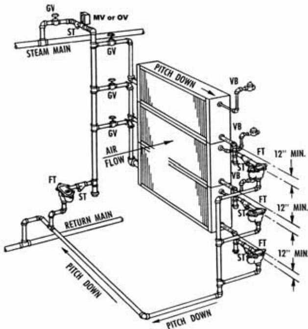
**Figure 53. Typical piping for Type NS steam coils and horizontal tubes for horizontal airflow**
