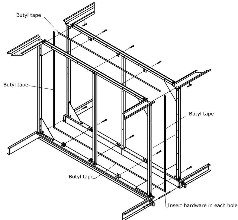
**Figure 23. Butyl tape is applied to shipping splits**
