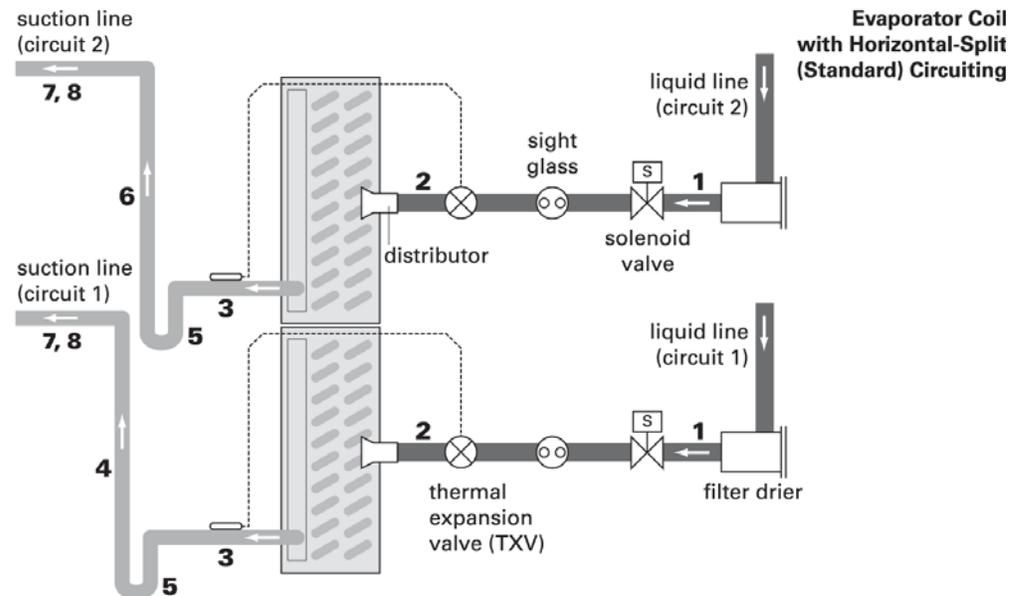
1. Pitch the liquid lines slightly—1 inch/10 feet [1 cm/3 m]—so the refrigerant drains toward the evaporator. See [Figure 63](#).
