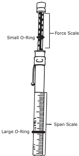
Check the fan belt tension at least three times during the first days of operation because there is a rapid decrease in tension until the belt settles in. To measure belt tension, use a belt tensiometer (see Figure 73). Determine actual deflection by depressing one belt with the belt tensiometer and measuring the deflection relative to the other belts or to belt line (see Figure 74). Adjust the belt tension to the correct pounds force and tighten all set screws to the proper torque.
