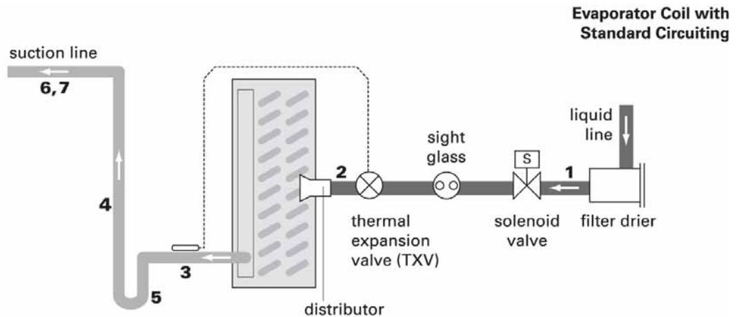
1. Pitch the liquid line slightly—1 inch/10 feet [1 cm/3 m]—so that the refrigerant drains toward the evaporator. See [Figure 60](#).
