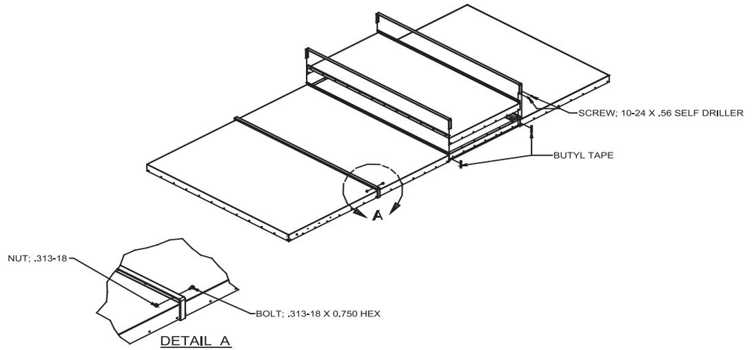
Figure 33. Trim roof joint strip
