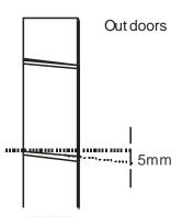
The hole must slope downwards towards the exterior. Note: Keep the drain pipe down towards the direction of the wall hole, otherwise leakage may occur.
