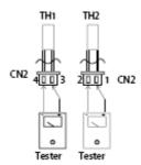
TH1: indoor room temperature sensor and outside air temperature sensor
