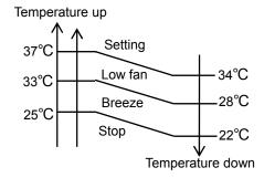
• In heating operation, if air conditioner turn off, the indoor fan motor will run most for 30
