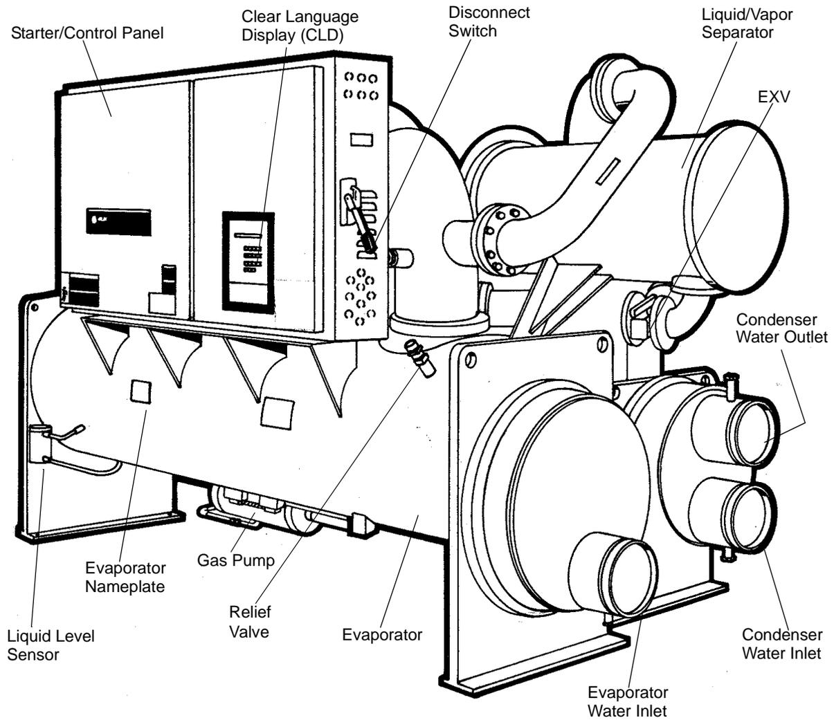
**NOTE:** The evaporator inlets and outlets are located opposite from those on the RTHA and RTHB units. The water inlet must be at the bottom of the shell for proper operation.
