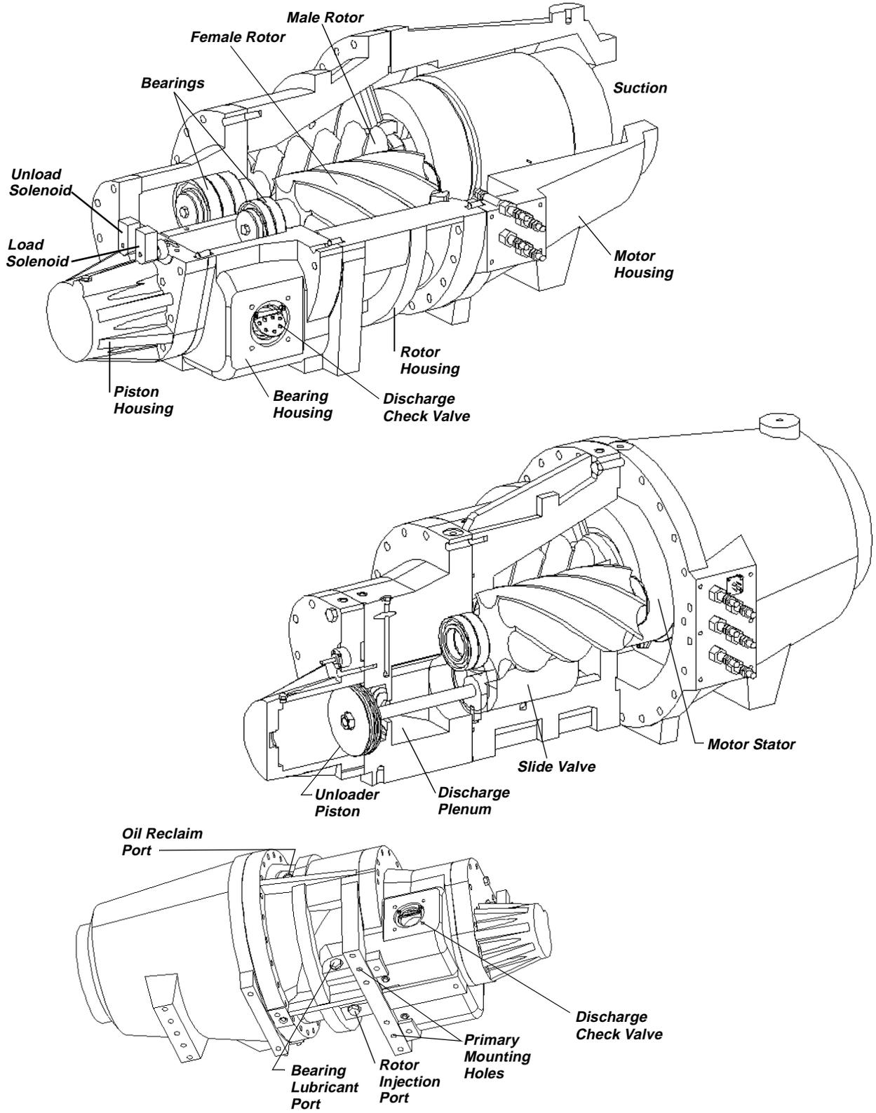
The compressor used by the Series R chiller consists of three distinct sections: the motor, the rotors and the bearing housing. Refer to *Figure 27*.
