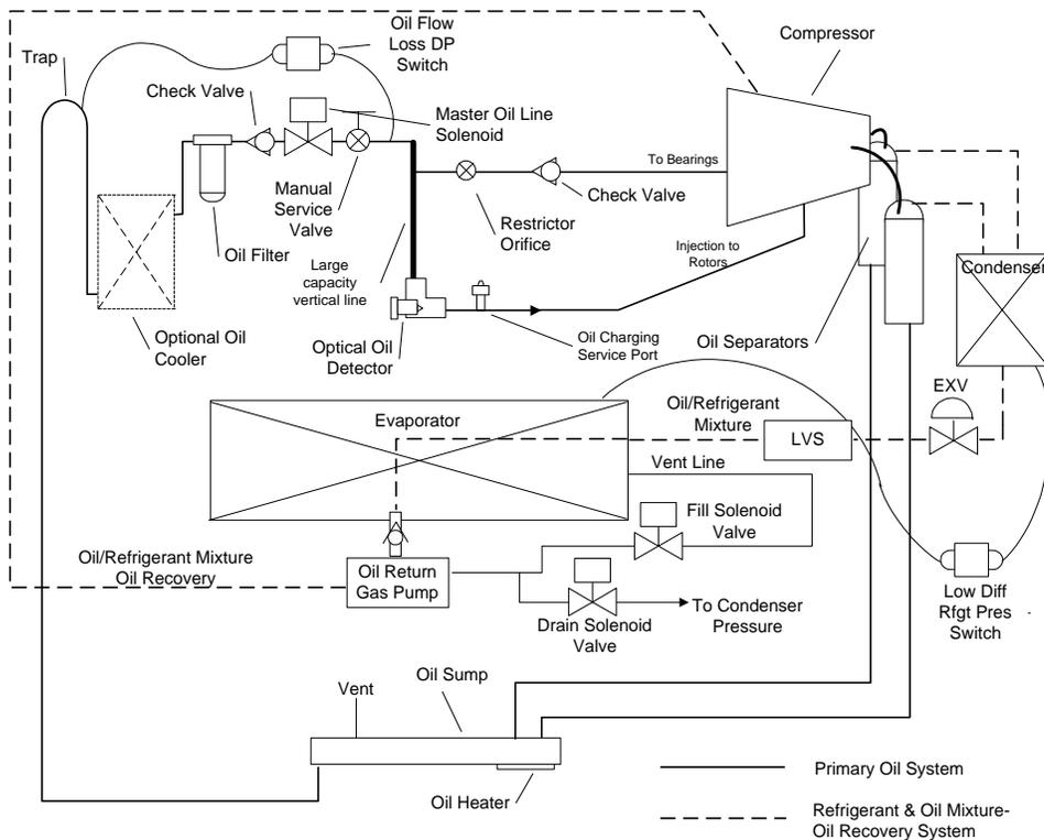
Oil that collects in the oil tank sump is at condensing pressure during compressor operation; therefore, oil is constantly moving to lower pressure areas.
