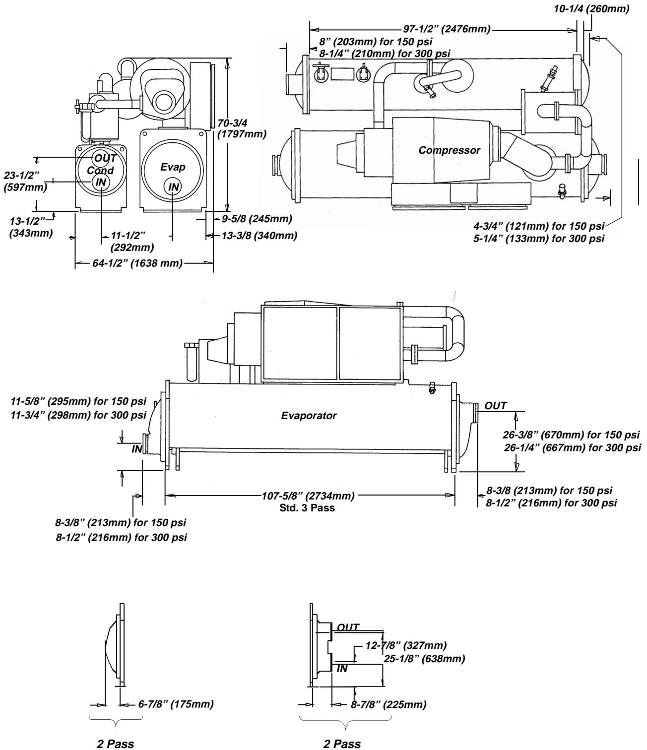
Figure 15 Condenser and Evaporator Water Connections - B1C1D1/B2C2D2
