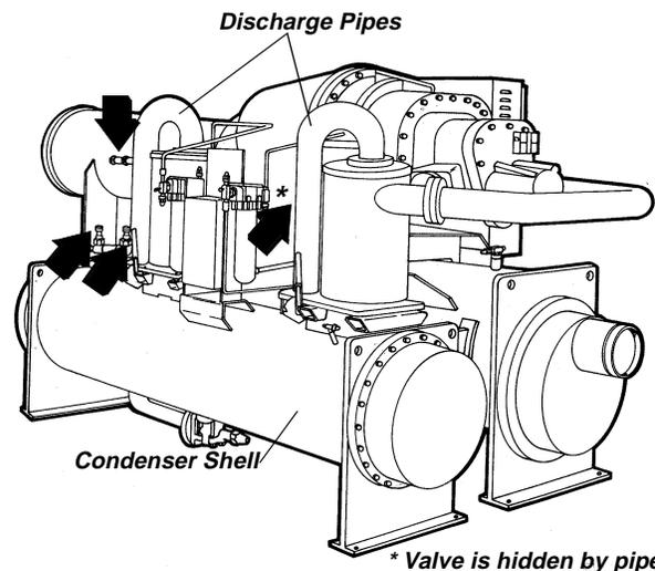
*NOTE: Once opened, relief valves tend to leak and must be replaced.*
