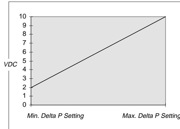
Condenser Pressure analog Output with “Delta” selected
