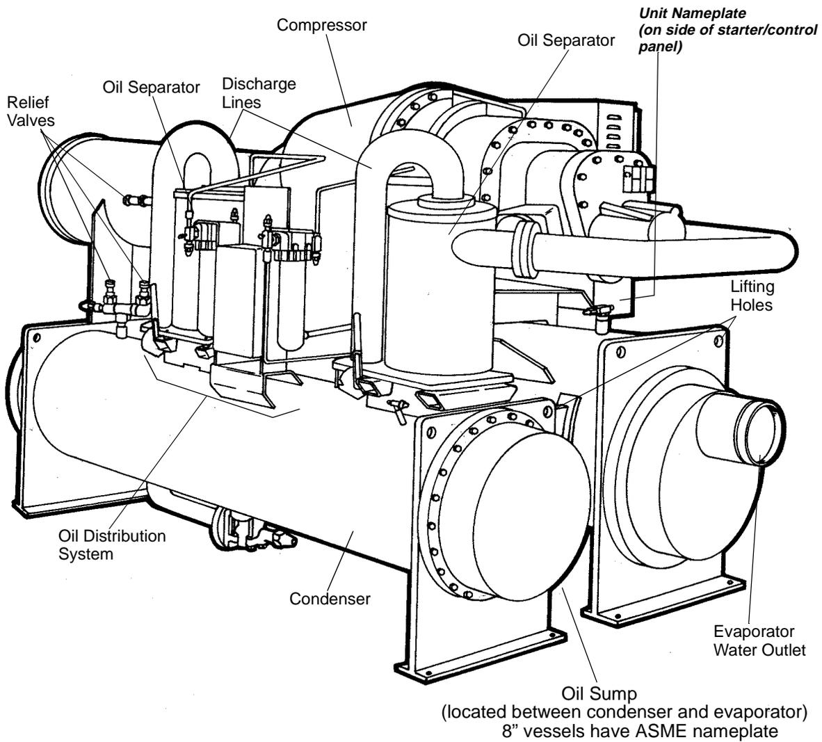
**NOTE:** The evaporator inlets and outlets are located opposite from those on the RTHA and RTHB units. The water inlet must be at the bottom of the shell for proper operation.
