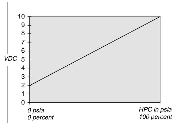
Condenser Pressure analog Output with “%HPC” selected
