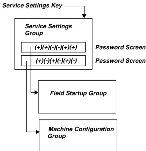
The other two groupings are protected, each with a separate password. These two groups are for changing parameters and settings for field commissioning and fundamental protection and control of the chiller subsystems (Service Set-up) or for programming of the UCM (machine configuration) if, for example, a UCM must be replaced.
