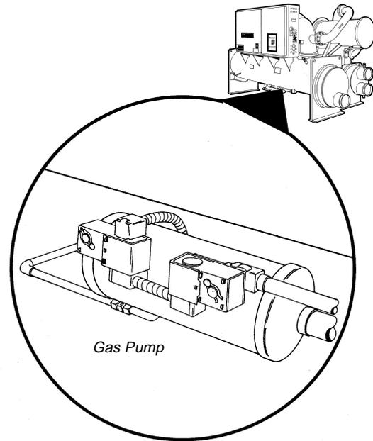
Despite the high efficiency of the oil separators, a small percentage of oil will get past them, move through the condenser, and eventually end up in the evaporator. This oil must be recovered and returned to the oil sump. The function of active oil return is accomplished by a pressure-actuated pump referred to as the “gas pump.”
