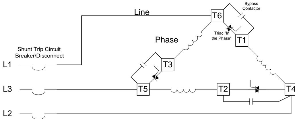
Note that even a Solid State Starter with its triacs “in the line” represent a similar hazard. Should a person contact any of the motor terminals, even with the motor off, the triac “off-state” leakage and finite snubber impedance would be enough to cause a severe, even fatal, electrical shock. In the case of the “in the phase” starter, the currents available could be quite high, as little or no impedance would be in series with the voltage source.
