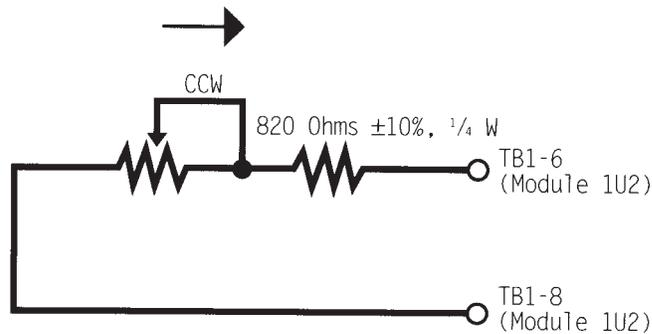
If the potentiometer is to be remotely mounted, it and the resistor must be connected to the UCM prior to mounting. Then, with the UCM display in Menu 0 and the display advanced to "Active Current Limit Setpoint", the UCM can be used to calibrate the positions of the potentiometer to correspond with the desired settings for the current limits. External resistor input values for various current limit setpoints are shown in Table 14.
