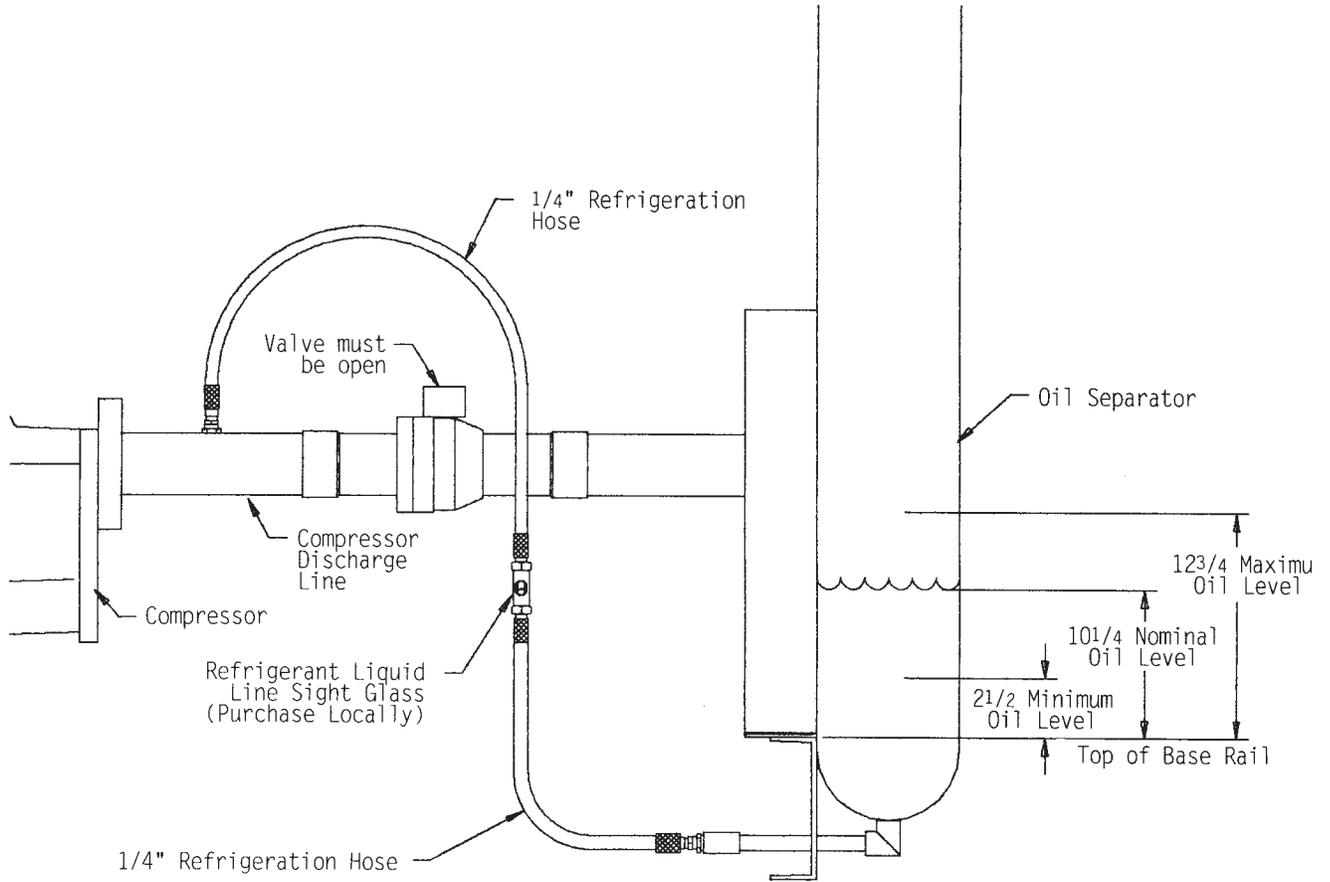
**Caution: Do not check oil level with machine operating. Severe oil loss will occur.**
