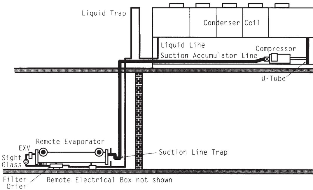
E. Horizontal portions of the suction lines must be downward sloping to the compressors. Suction lines must be insulated.
