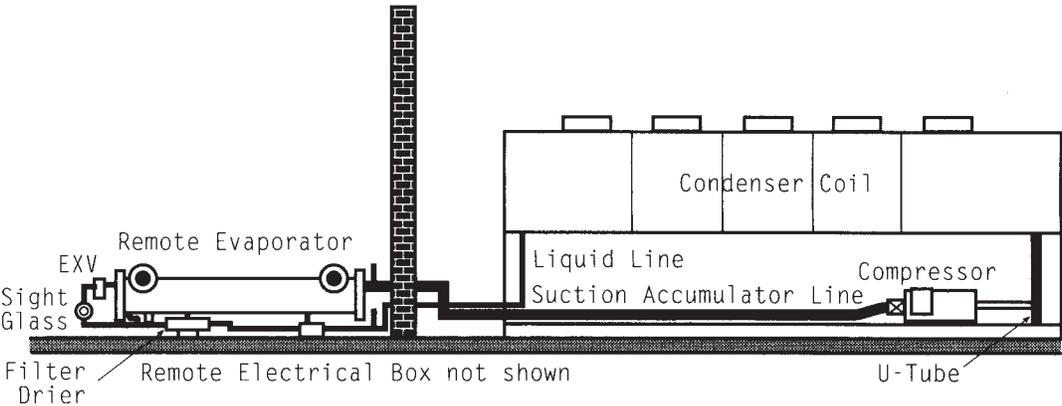
A. The line sizes established in this installation manual are to be used only for 40-50 F leaving water temperature and full-load ice-making applications.
