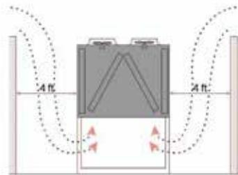
The RTAC has the smallest recommended side clearance on the market: 1.13 meters (4 feet) to maintain maximum performance. In locations where space is further limited and airflow is restricted, the RTAC will remain operational.
