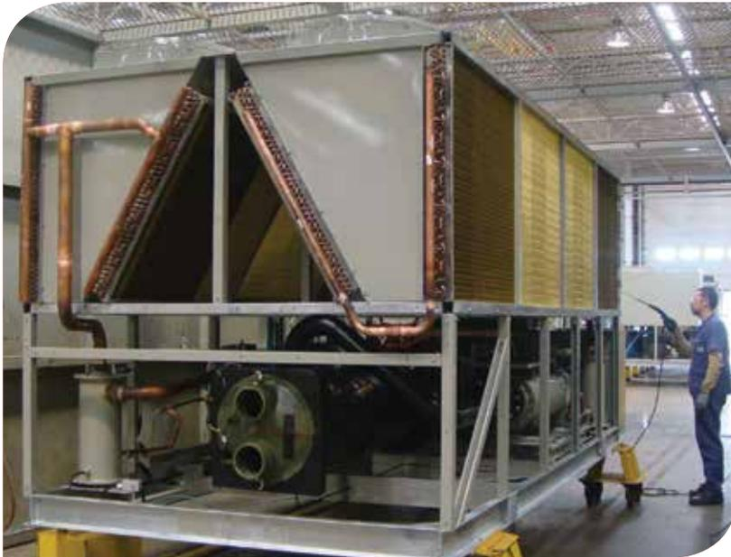
Trane units and compressors are extensively tested in order to ensure robust operation and smooth starting.
