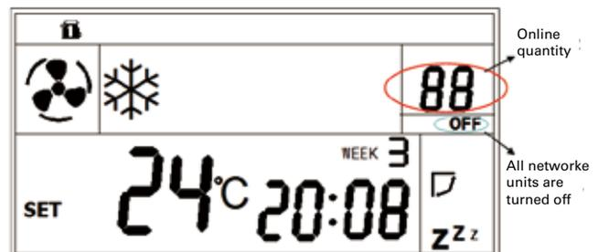
Notes: A. If the online quantity displayed is inconsistent with the actual quantity, inspect whether the connecting line is connected correctly, or confirm whether the unit dial code is correct.
