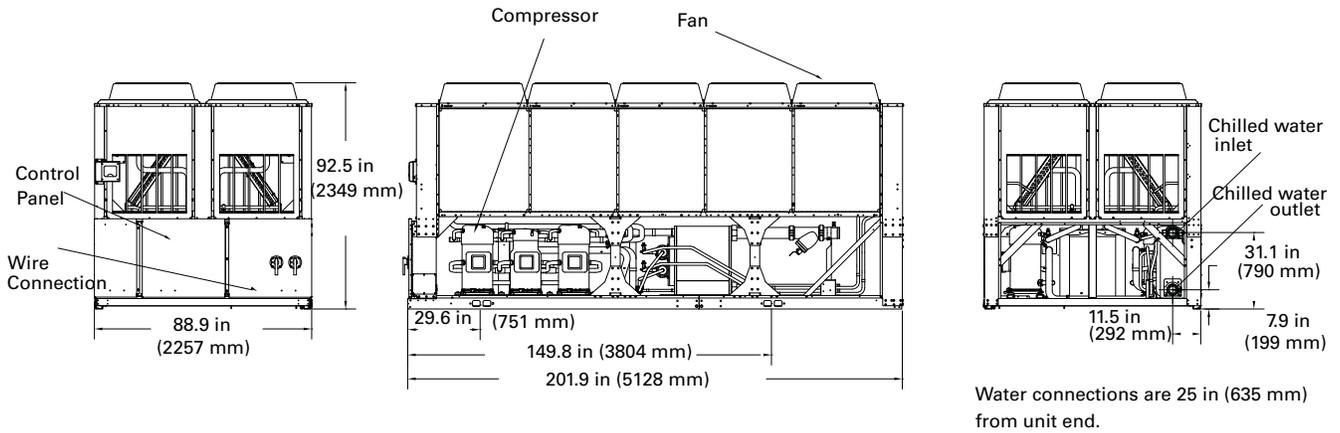
Figure 17. CGAM 130 ton- service clearances and mounting locations
