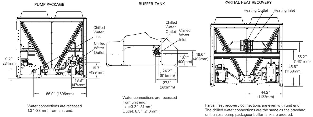
**Figure 29. CGAM 80 -130 ton — pump package, buffer tank, partial heat recovery unit water connections<sup>(a)</sup>**
