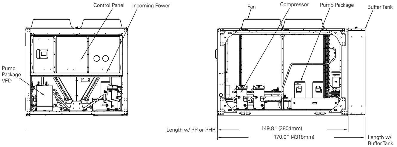
**Figure 22. CGAM 80 and 90 ton — pump package, buffer tank, partial heat recovery**
