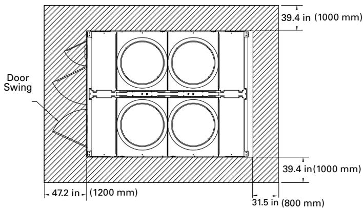
More clearance may be needed for airflow depending on the installation.
