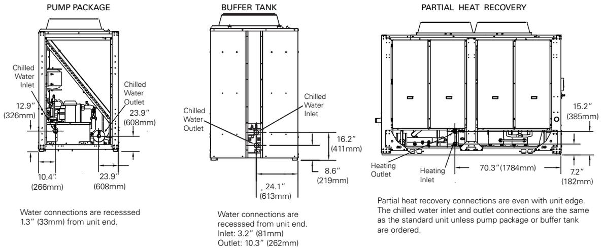
**Figure 26. CGAM 30 and 35 ton — pump package, buffer tank, partial heat recovery unit water connections**
