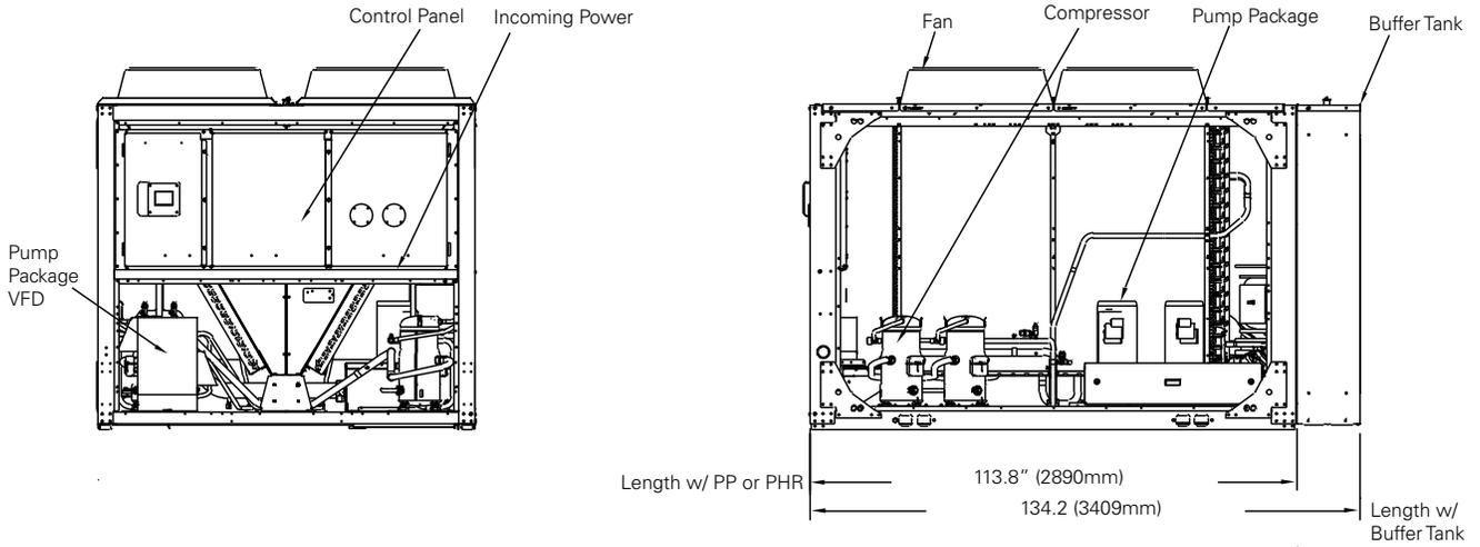
**Figure 21. CGAM 60 and 70 ton — pump package, buffer tank, partial heat recovery**
