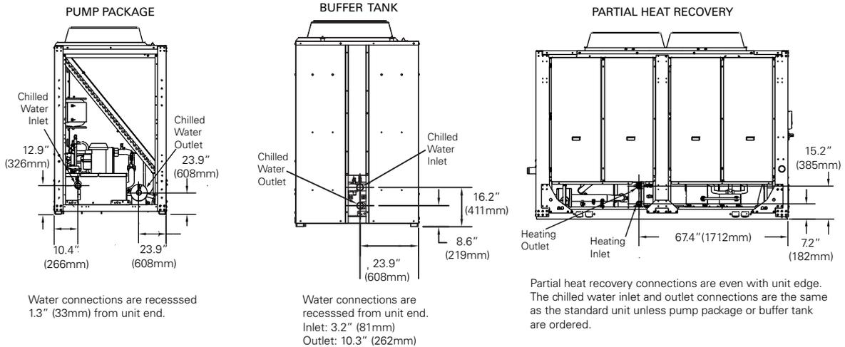
**Figure 27. CGAM 40 and 52 ton — pump package, buffer tank, partial heat recovery unit water connections**
