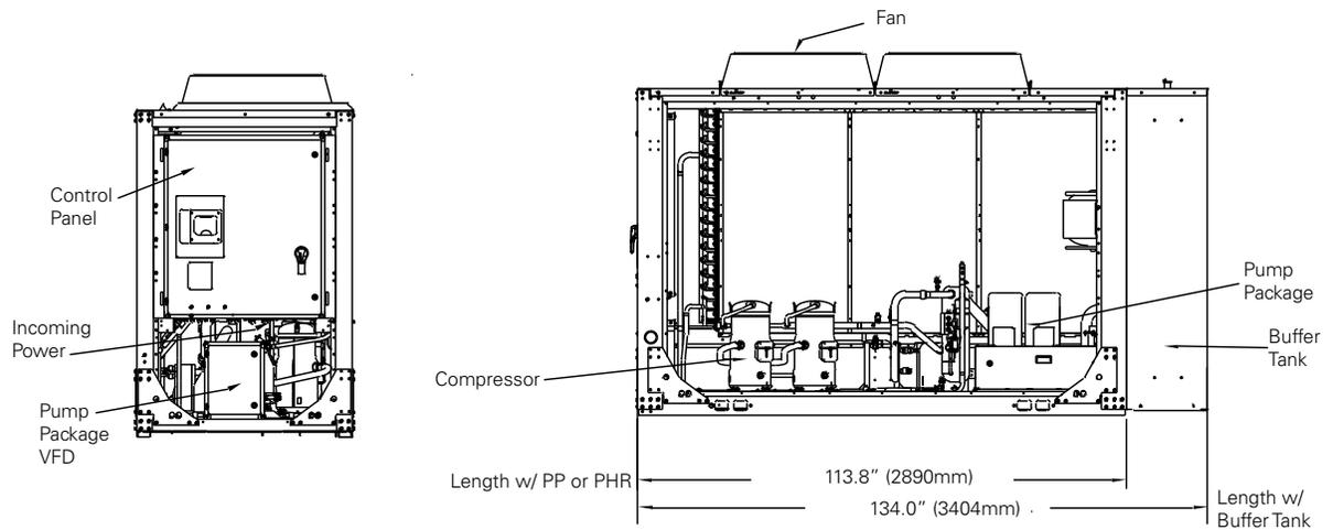
Figure 19. CGAM 30 and 35 ton — pump package, buffer tank, partial heat recovery
