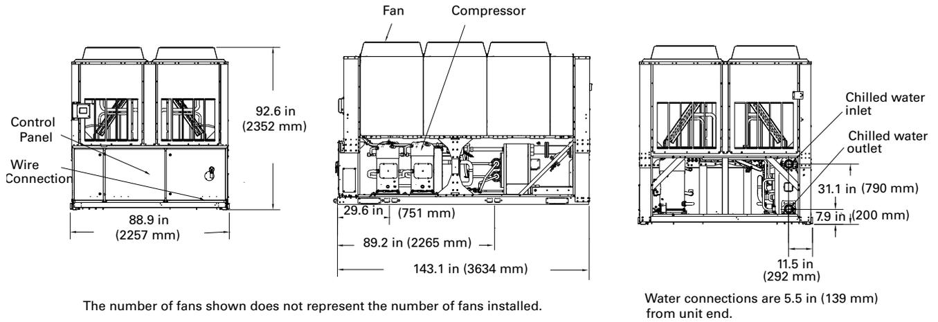
Figure 13. CGAM 80 and 90 ton - service clearances and mounting locations
