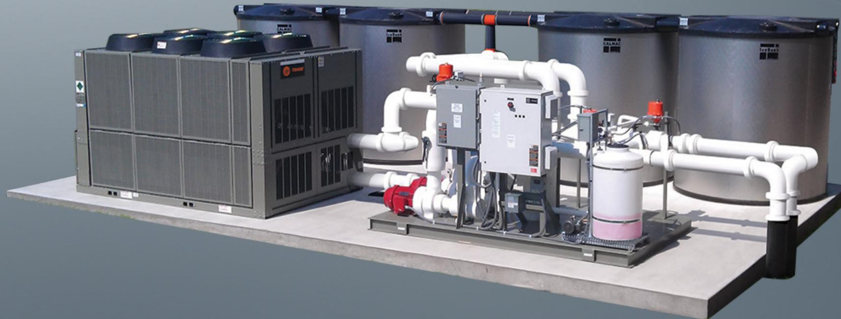
The Trane Thermal Battery system is a Trane controlled chiller plant enhanced with **thermal energy storage**. The chiller plant operates like a battery, charging Ice Bank® energy storage tanks when excess or inexpensive energy is available. And discharging when demand is high or price is high or when the utility asks for the discharge to occur.
