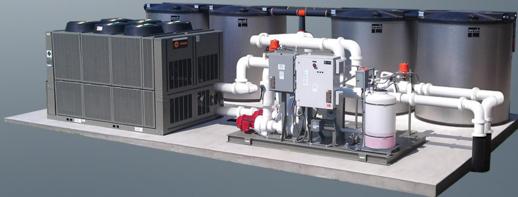
The Thermal Battery™ system features a standard chiller with ice making controls as factory option, completion module with pumps, controls, control valves, PFHX, if needed and all piping specialties. The control system dash boards demonstrate savings, modes of operation, schematics and much more. And of course thermal energy storage equipment.
