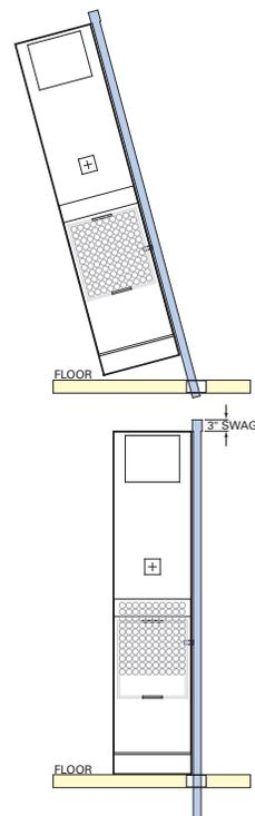
If unit cabinet assembly includes *factory provided risers*, and "no" field provided between-the-floor riser extensions, please move to [Step 1](#).
