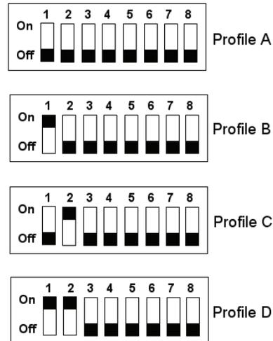
**Note:** Units with the optional ECM with deluxe 24V or Tracer® ZN510 controls are shipped from the factory on Profile B.
