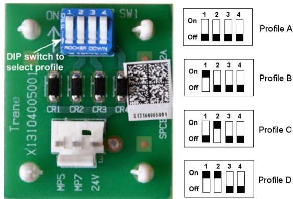
Installations at altitudes above 2000 feet may require an adjustment to the fan speed setting to achieve the proper airflow. To adjust the airflow to get the desired CFM, set the DIP switches located in the control box to the proper profile setting. Tracer® TU can be used to make further adjustments to the fan speed.
