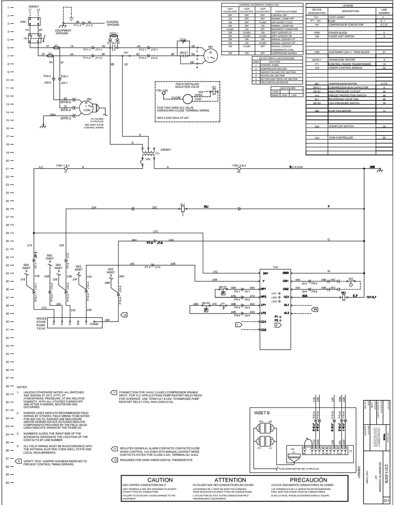
Figure 24. Tracer® UC400-B with ECM
