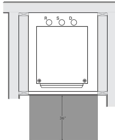
(a) Clearance shown is at unit front for chassis removal.
