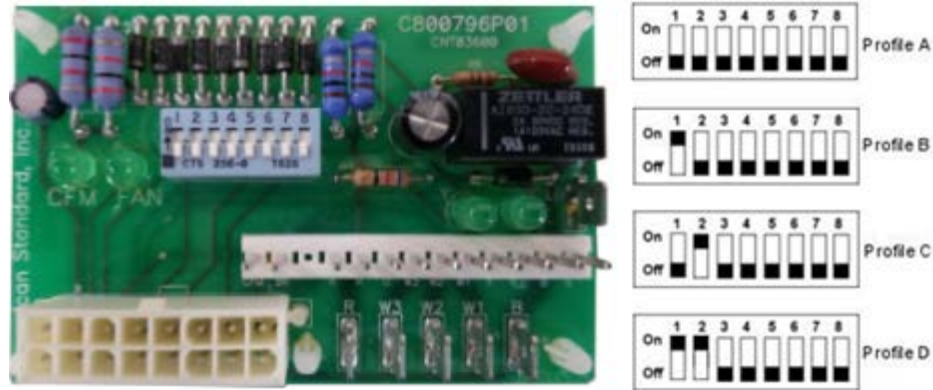
Figure 12. ECM control board
