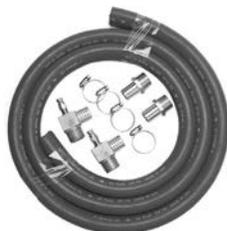
The pump module hose kit consists of two brass, 3/4 in. or 1 in., male pipe thread (MPT)-by-barb fittings; two brass 90° 1-inch, MPT-by-barb elbows with pressure/temperature ports; and 10 ft of rubber hose with 4 hose clamps. The pump module hose kit is available separately from the pump module.
