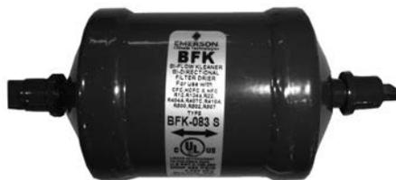
The filter drier is a solid core, bi-directional, liquid line filter drier for heat pump applications. Internal check valves allow flow and filtration in either direction.
