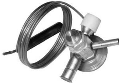
The refrigerant flow metering is made through the thermal expansion valve (TXV). It allows the unit to operate with an entering fluid temperature from 25°F to 120°F and entering air temperatures from 50°F to 95°F. The valve is designed to meter refrigerant flow through the circuitry to achieve desired heating or cooling.
