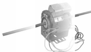
The supply-air (blower) motor is a multi-speed motor with internal thermal overload protection. The motor bearings are permanently lubricated and sealed. Standard motors are rated from 220 CFM at low speed (unit size 006) to 530 CFM at high speed (unit size 018).
