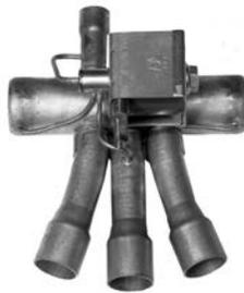
A system reversing valve (4-way valve) is included with all heating/cooling units. This valve is piped to be energized in the cooling mode to allow the system to provide heat if valve failure were to occur. Once the valve is energized for cooling, it will remain energized until the control system is turned to the OFF position, or a heating cycle is initiated.
