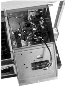
Controls for the console unit are housed on the right-hand side of the chassis. The box dwells above the refrigeration section of the chassis.
