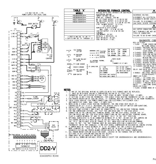
/ WARNING DISCONNECT ALL ELECTRICAL POWER INCLUDING REMOTE DISCONNECTS BEFORE SERVICING. FAILURE TO DISCONNECT POWER BEFORE SERVICING CAN CAUSE SEVERE PERSONAL INJURY OR DEATH. USE COPPER CONDUCTORS ONLY! UNIT TERMINALS ARE NOT DESIGNED TO ACCEPT OTHER TYPES OF CONDUCTORS. FAILURE TO DO SO MAY CAUSE DAMAGE TO THE EQUIPMENT DIAGNOSTIC CODES
