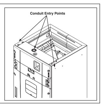
**STEP 3** - Route conduit (if used) to the entry point and connect.
