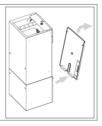
**STEP 3** - Remove the control board from the control pocket by sliding the control pocket mounting plate out until the first stop is reached.
