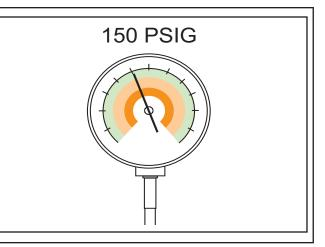
**STEP 9** - Check for leaks by using a soapy solution or bubbles at each brazed location.
