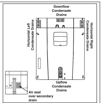
**Note:** A small amount of sealant must be applied around the drain line(s) passing through the panel to prevent air leakage and possible water drips.
