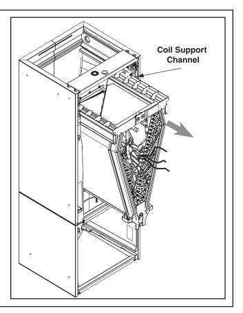
**STEP 7** - Use a 5/16 Allen wrench on the locking mechanism on each side of the bottom half of the cabinet to loosen the locking mechanism. The locks loosen by turning counter-clockwise approximately 3/4 of a turn.
