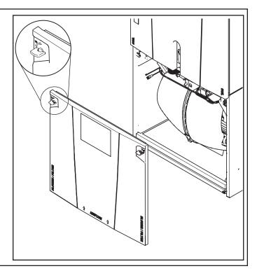
The Coil, Line Set, and Heater panels are removed using Phillips head screws.
