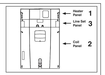
*Important:* Do NOT unseal coil refrigerant connection stubs until ready to make connections.
