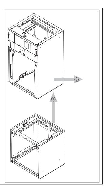
**STEP 9** - For extremely tight spaces where the cabinet needs to be rotated through a small opening, remove the top panel and all cross members. Use a manual driver to avoid stripping screw holes.
