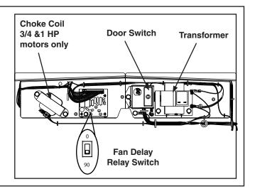
**STEP 2** - Reinstall all panels before starting the air handler.
