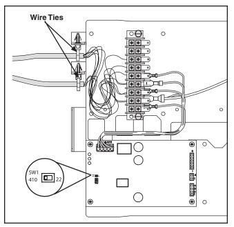
**STEP 7** - Slide control plate assembly into the control pocket until fully seated. The control plate should be flush with the outer edge of the unit.
