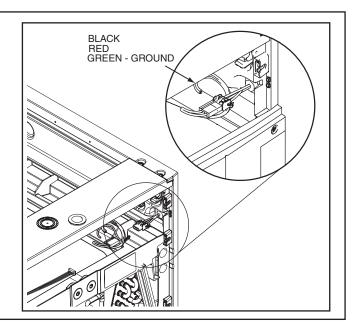
**STEP 5** - If the L1, L2, and ground wires enter the case from the left side, use a field supplied 1/2"-5/8" maximum length screw and wire tie to hold the wires to the top center of the Heater Compartment.
