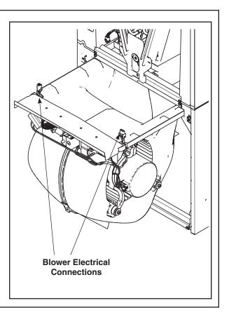
**STEP 2** - Disconnect the two wiring connections routed to the blower assembly.
