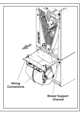
**STEP 4** - Remove airflow diverter from the bottom of coil drain pan by gripping the plastic diverter, using your thumbs to spread the top of the diverter slightly outwards, and then pulling down and out through the blower opening as illustrated.
