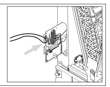
**STEP 8** - Replace Coil panel making sure that the wires are located within the wire pass-through provided in the panel.
