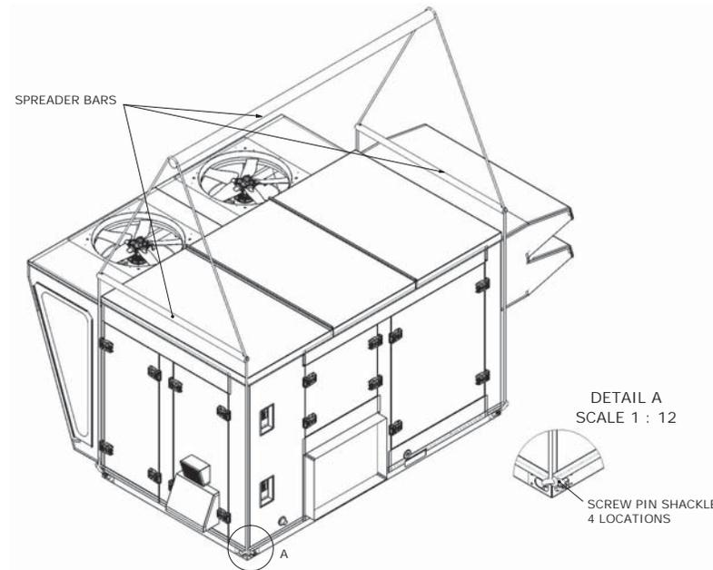
**Figure 36. Four-point lift (OAD cabinet with exhaust fan and no ERV)**
