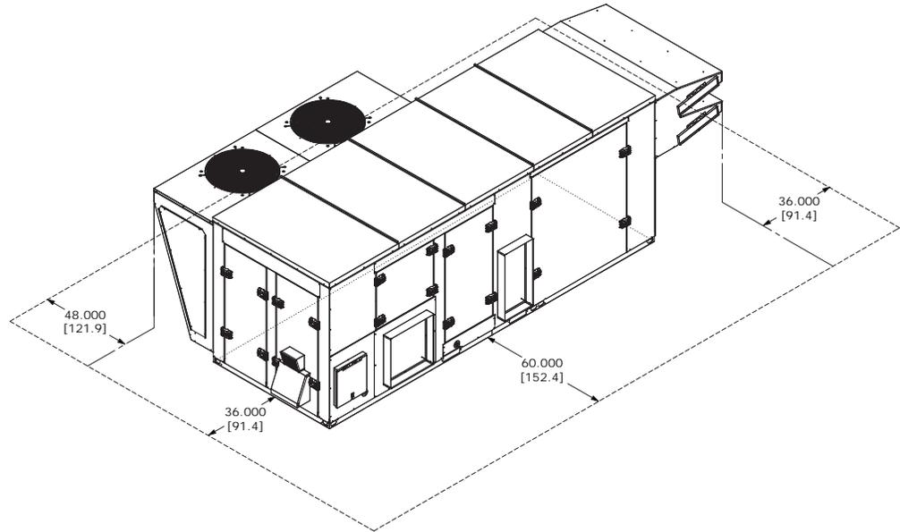
Note: 72 in. (182.9 cm) clearance is required above the condenser fans.
