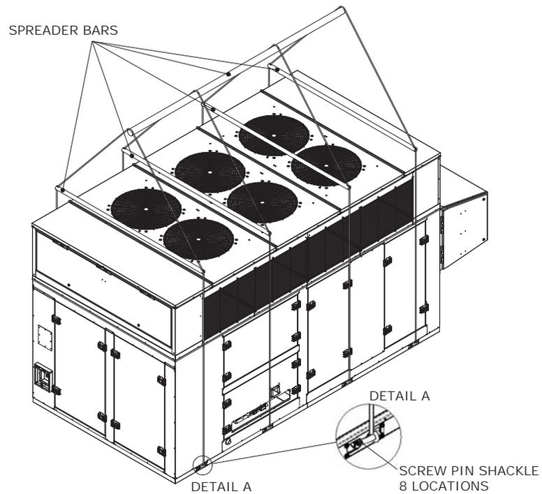
**Figure 39. Ten-point lift (OAN cabinet with exhaust fan and no ERV)**
