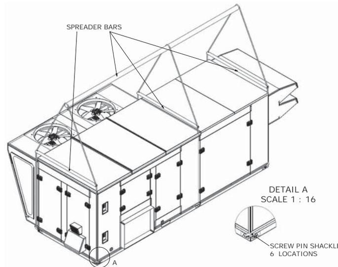
**Figure 38. Eight-point lift (OAN cabinet with no exhaust fan or ERV)**
