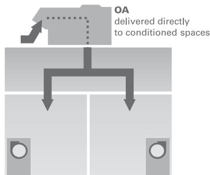
**Figure 3. Indirect discharge to fan-coil units**
