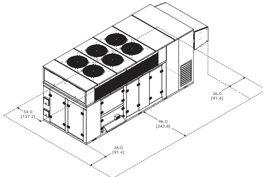
Note: 72 in. (182.9 cm) clearance is required above the condenser fans.
