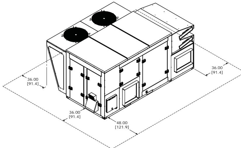
Note: 72 in. (182.9 cm) clearance is required above the condenser fans.
