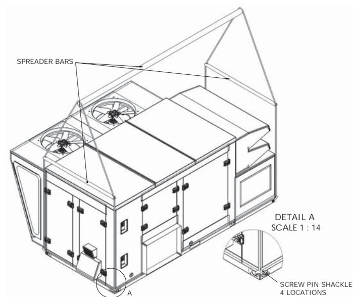
**Figure 37. Six-point lift (OAD cabinet with ERV section)**
