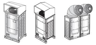
Examples of condenser air discharge ducts
