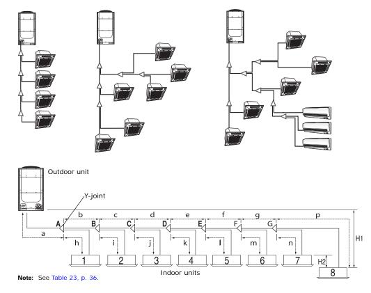
Figure 16. Single installation with distribution header: Heat pump
