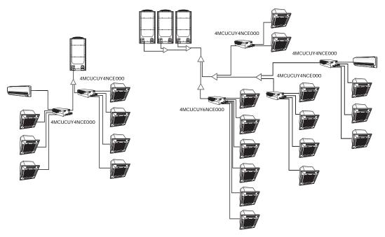
Figure 22. Single installation with MCU: Heat recovery
