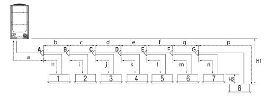
Use Table 8 to determine the diameter of the main pipe. If distance a+b+c+d+e+f+g+p > 295.3 ft, the main pipe (A in Figure 10) must be upsized.
