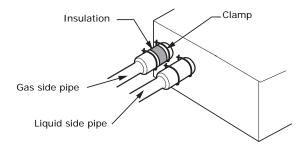
4. Cut off excess insulation.
