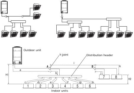
Figure 17. Single installations with Y-joint and distribution header: Heat pump
