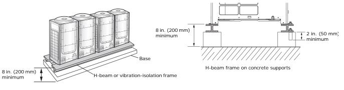
After installing a vibration-isolation frame:
