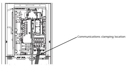
Figure 29. Communications cable clamping location
