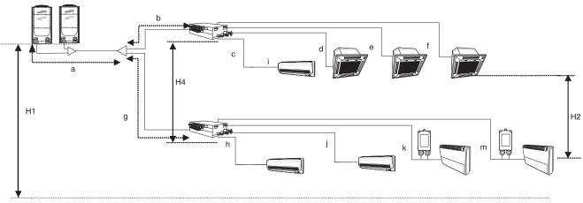
Figure 23. Module installation with MCU and Y-joint: Heat recovery
