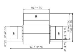
A: Optional condenser air discharge duct B: Optional wind/snow protection duct
