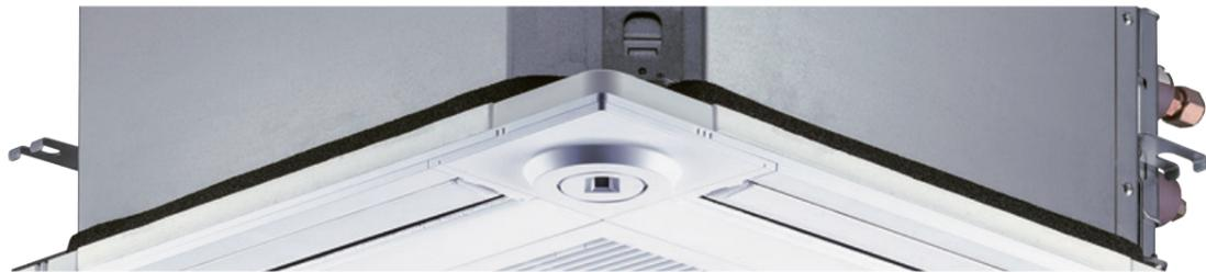
The 3D i-see Sensor detects the number of occupants in a room and adjusts the temperature accordingly, making automatic energy-saving operation possible in places where the number of occupants frequently changes. Additionally, when the area is continuously unoccupied, the system switches to an enhanced power-saving mode.
