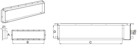
Fig.9 Air Supply Outlet
