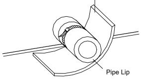
Fig.13 Thermal Insulation of the Condensate Pipe
