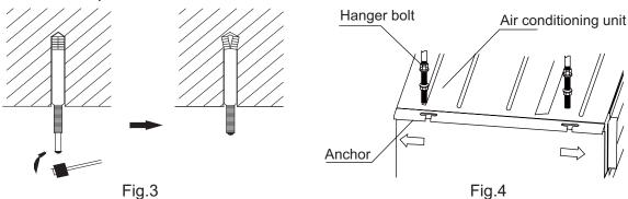
Install the hanger on the indoor unit, as shown in Fig.4. Install the indoor unit on the ceiling, as shown in Fig.5.
