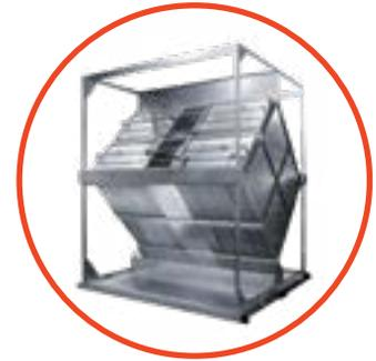
**Air-to-air plate heat exchangers** are a great solution to recover sensible energy (heat only) from an exhaust air stream, with little or no cross-contamination. These exchangers may also be used for free reheat in dehumidification applications, including dedicated outdoor air systems. Where exhaust air is not available, exchangers can be used in series to heat the dehumidified air.
