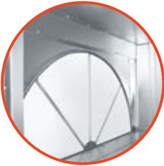
**AHRI 1060–certified energy wheels** recover energy from the exhaust air stream, transferring it to the air being distributed throughout a building and reducing the workload on chillers and boilers, lowering energy use and utility bills. Energy wheels are available in both indoor and outdoor arrangements, and can be applied in both a 100 percent outdoor air unit and a mixed air unit. Trane energy recovery software can model your specifications to show the benefit of payback analysis.
