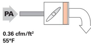
**VAV terminal with 40% minimum airflow setting**
