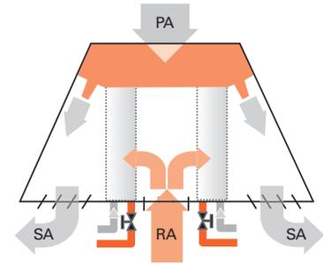
For this same example office space, the design airflow delivered by a conventional VAV system would be 0.90 cfm/ft<sup>2</sup>. At design cooling conditions, primary airflow required for the ACBs serving this space is 60 percent less than for the conventional VAV system. However, this does not translate to a 60 percent reduction in fan energy use, as will be discussed later in this EN under the *claimed advantage 3* section.
