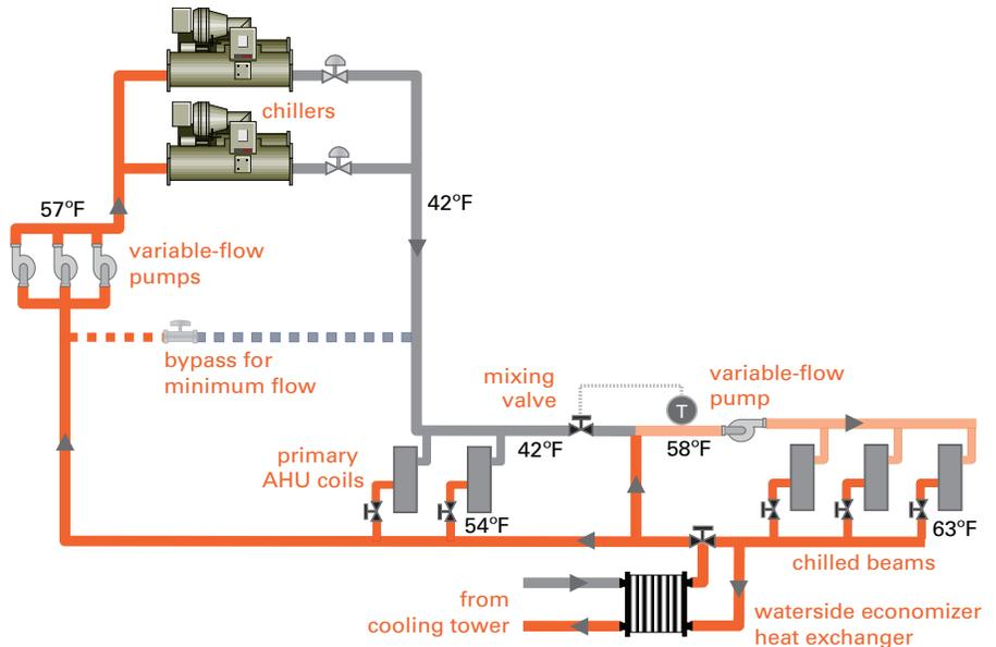
Note: Other plant configurations have been used—such as putting the primary AHU coils and chilled beams in series or putting chillers in series and diverting some of the warmer water leaving the upstream chiller to serve the chilled beams—and they can provide energy benefits over this example configuration, but they also increase complexity.
