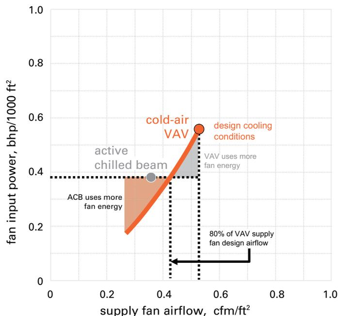
Note: For the cold air VAV system (48°F primary air, rather than conventional 55°F), assumes the ductwork has been downsized for first cost savings—so total static pressure remains the same at 4 in. H<sub>2</sub>O—and assumes 60% fan efficiency.
