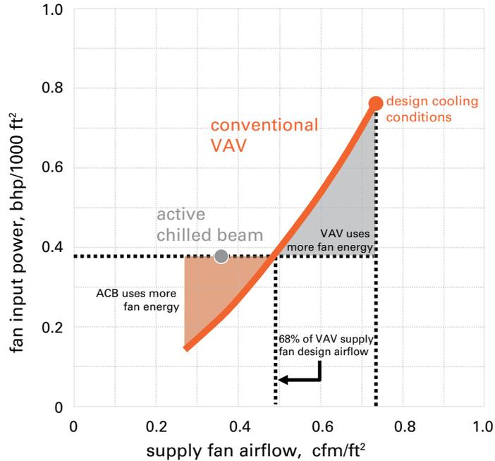
Note: For the ACB system, assumes total static pressure 4 in. H<sub>2</sub>O and 60% fan efficiency:  $bhp = (0.36 \text{ cfm/ft}^2 \times 4 \text{ in. H}_2\text{O}) / (6356 \times 0.60) = 0.00038 \text{ bhp/ft}^2$  or 0.38 bhp/1000 ft<sup>2</sup>. For the VAV system, see Table 2. The VAV fan input power levels off below 0.27 cfm/ft<sup>2</sup>, assuming all VAV terminals are at the minimum airflow setting, 30% of design zone airflow (0.30 x 0.90 cfm/ft<sup>2</sup> = 0.27 cfm/ft<sup>2</sup>).
