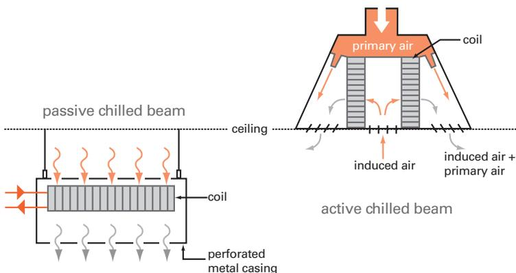
Figure 2. Examples of active chilled beams
