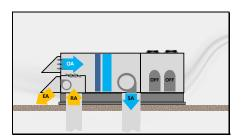
However, when the conditions are right, this outdoor-air damper opens further to bring in more outdoor air, reducing the need to operate compressors to provide cooling.
