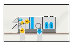
As you can see, typical operation includes the use of mechanical cooling while bringing in minimum outside air quantities.
