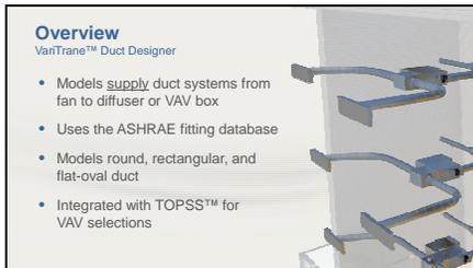
Duct Designer will model supply duct systems from the main fan all the way to the diffuser or VAV box. It's important to note that this software is used to design supply ducts, not return ducts.
