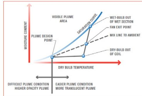
Cooling tower cold-weather condensation plume
