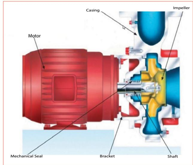
Typical centrifugal pump package cutaway
