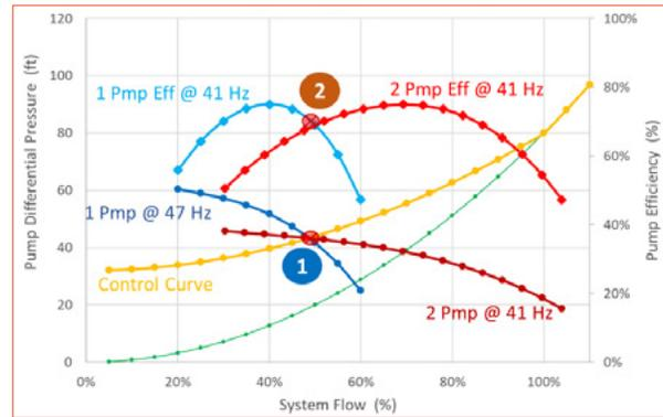
Efficiency-based pump staging
