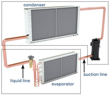
A split system consists of three primary components:
