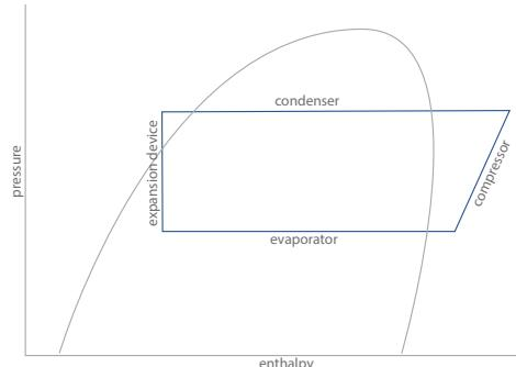
at normal temperatures) will evaporate and expand to produce a cooling effect.
