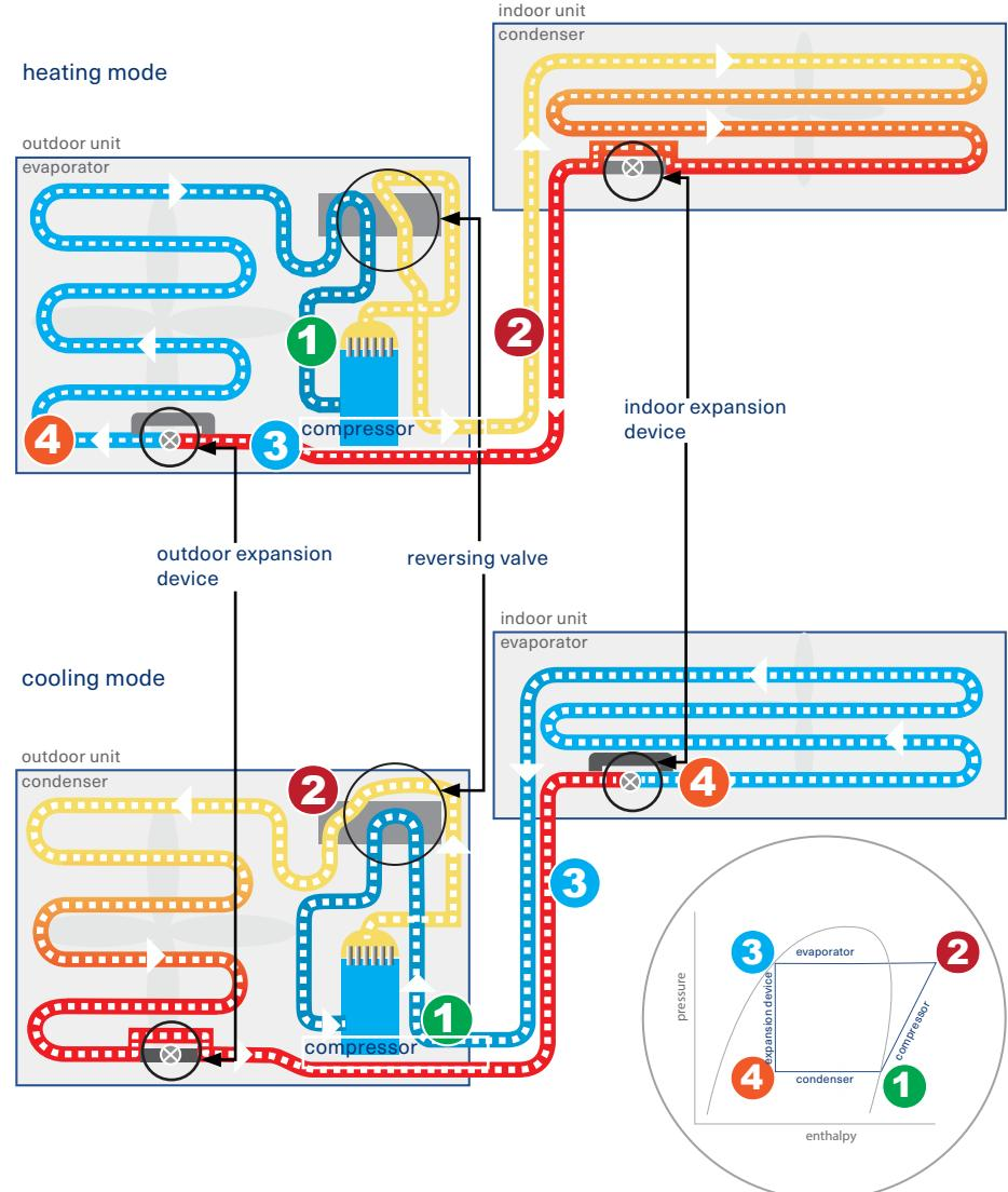
An ODU designed to operate as a heat pump will look similar to an ODU setup to operate as an air conditioner. The primary difference is that the ODU will include two additional components (Figure 4):
