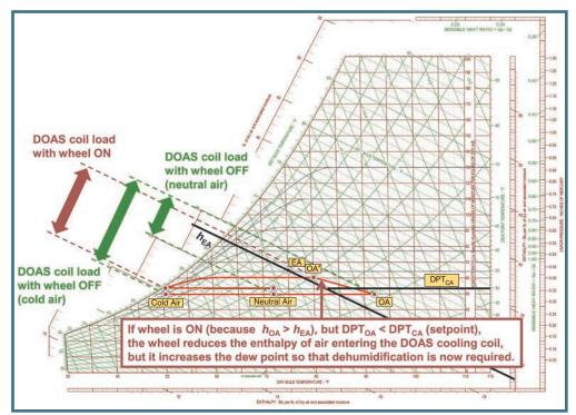
Figure 5: Total energy wheel control on a hot, dry day.
