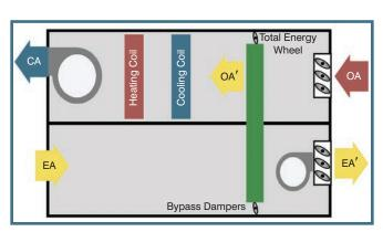
Figure 1: Exhaust-air energy recovery in a dedicated OA system.
