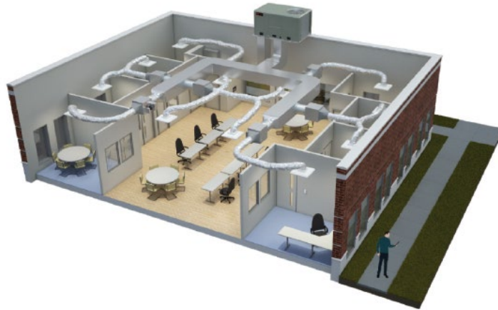
Figure 1. Example of a small commercial building served by a packaged rooftop unit
