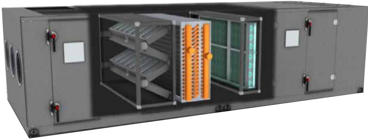
Viruses, odors, VOCs and micro-organisms pass through the filter and into the TCACS' ultraviolet germicidal irradiation (UVGI) area, where they are exposed to a high-intensity ultraviolet light. This UV radiation penetrates micro-organisms such as fungi, bacteria and viruses and damages their DNA bonds, sterilizing them.
