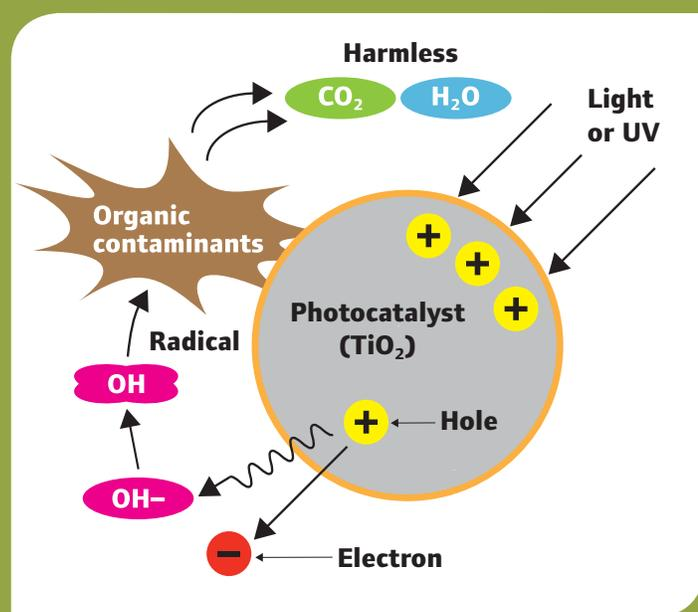
UV photons energize a photocatalyst media panel creating highly reactive hydroxyl radicals. Hydroxyl radicals convert organic compounds into simpler compounds and ultimately into water ( $\text{H}_2\text{O}$ ) and carbon dioxide ( $\text{CO}_2$ ).
