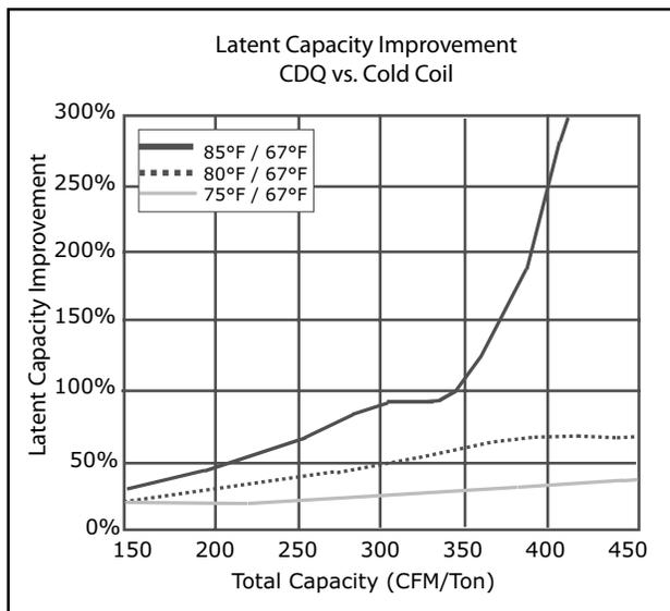
The improvement in latent capacity makes a CDQ system beneficial not only in low dew point applications but also in comfort cooling applications, especially at part load conditions. For example, at 400 cfm/ton, the CDQ system will remove 70 percent more water vapor from 80°F/67°F air than a cooling coil would remove by itself.
