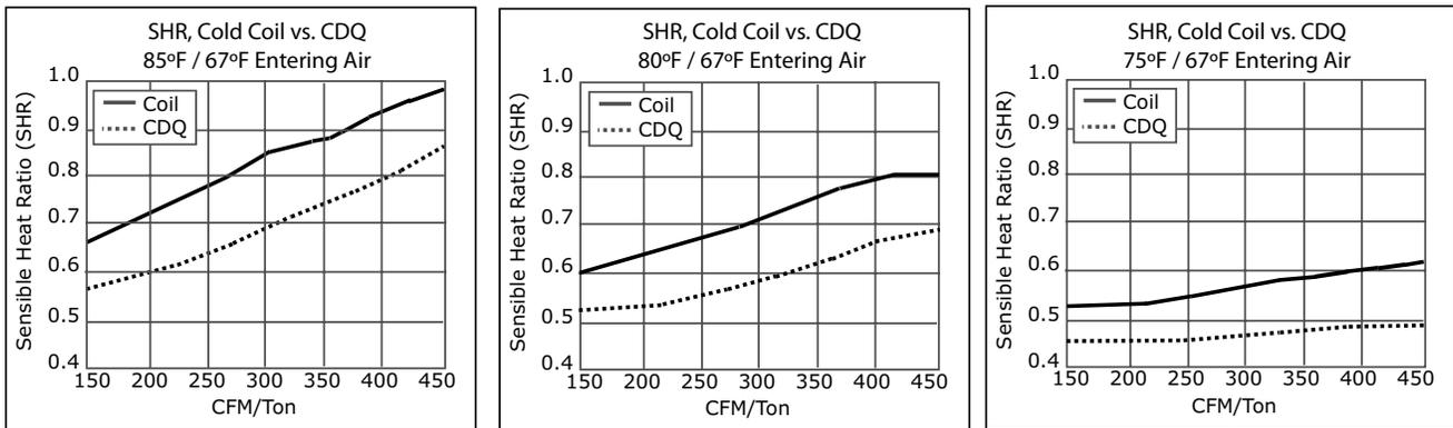
This reduction in unit SHR is not accomplished by adding heat. It is a result of increasing the latent capacity of the coil with the CDQ wheel. This increase in latent capacity is achieved without increasing the total capacity. Figure 13 is the same data represented in terms of latent capacity improvement. The latent capacity improvement at the examples conditions range from 15 to 550 percent.
