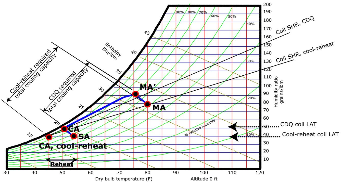
The cooling coil SHR, sensible heat ratio (the ratio of sensible cooling to total cooling), is also lowered with a CDQ system without using reheat. This helps the unit better match building loads, especially during part load conditions and reduces the need of reheat. The temperature gain from the wheel is minimal, typically 3°F to 9°F, thus the system can cool and dehumidify.
