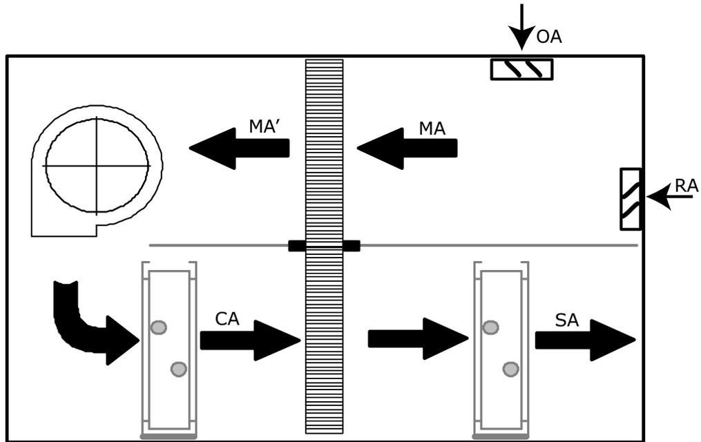
Most applications of the CDQ air handler will have components configured as described in the previous examples: outside air and return air inlets, filter, wheel pass one, supply fan, cooling coil, wheel pass two, then optional reheat coil.
