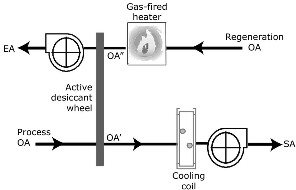
Depending on the required dew point of the process air, regeneration air temperatures typically range from 150°F to 300°F. The warmer the regeneration air ( $OA''$ ) is, the drier the resulting process air ( $OA'$ ) will be.
