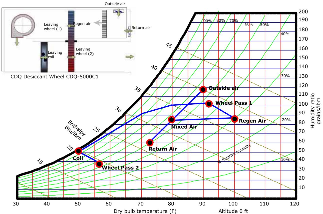
Table 1 shows an example of the condition in Figure 17 and how it can be achieved in three different ways. In this example, a CDQ system with preheat requires the most cooling capacity, but the temperature leaving the cooling coil is the warmest. Preheat can be modeled and predicted with Trane CDQ Performance Software.
