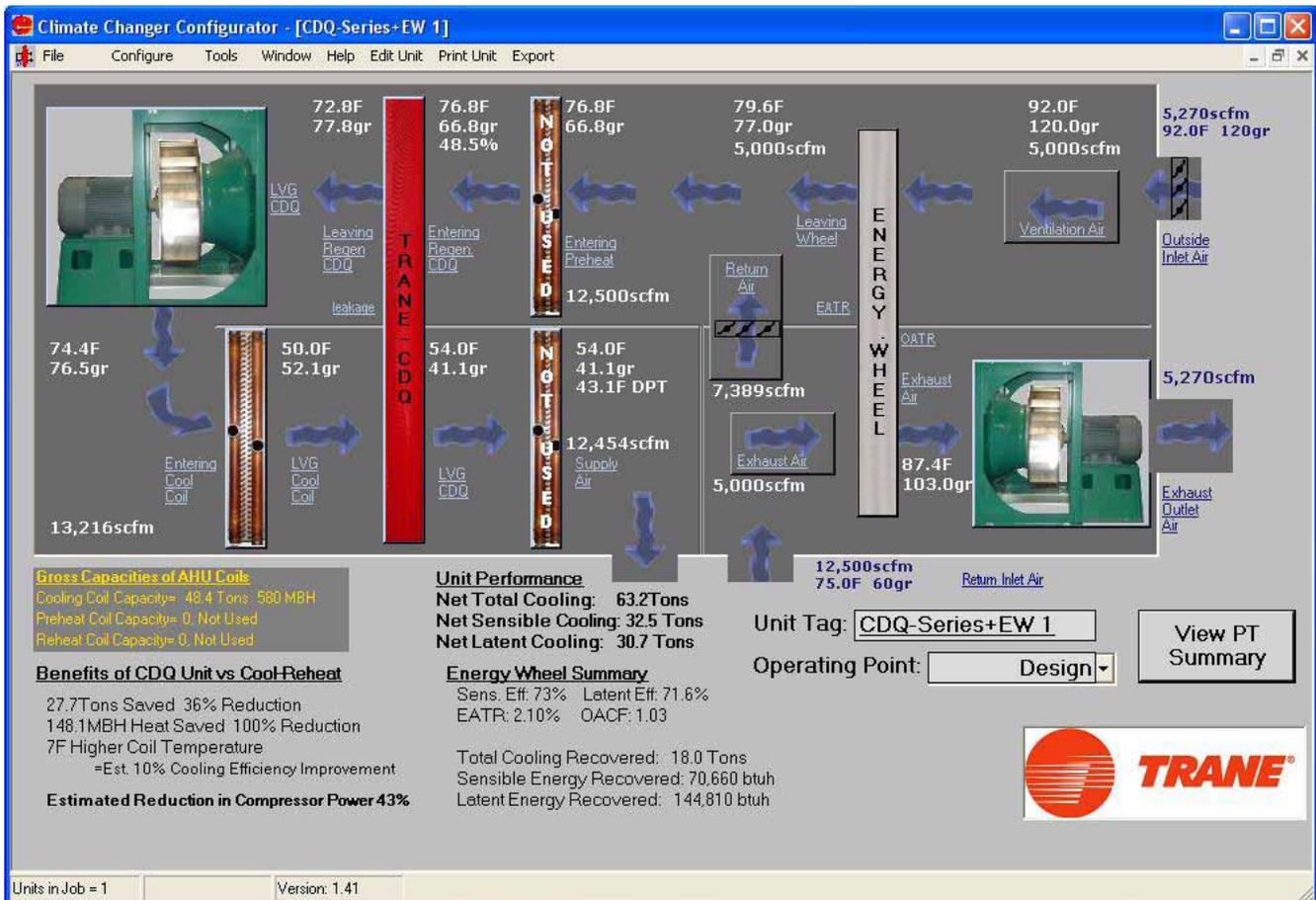
Figure 23. CCC summary for CDQ output for dehumidification design conditions
