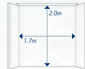
Trane HSWA can easily fit through a set of standard double doors.
