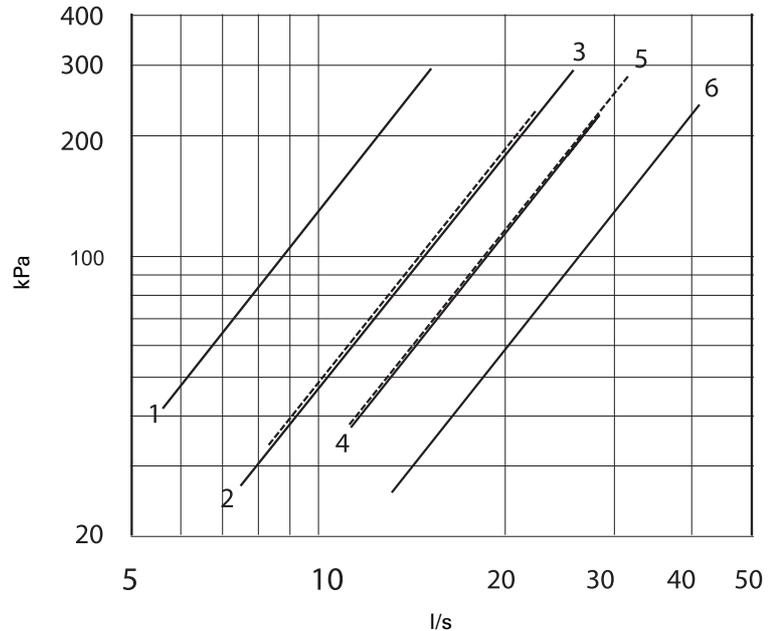
**Figure 14 - Water Pressure Drop RTAD Free Cooling - Free Cooling Mode**
