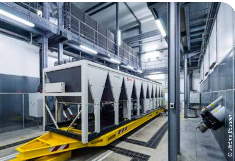
Sintesis unit RTAF 310T under test
