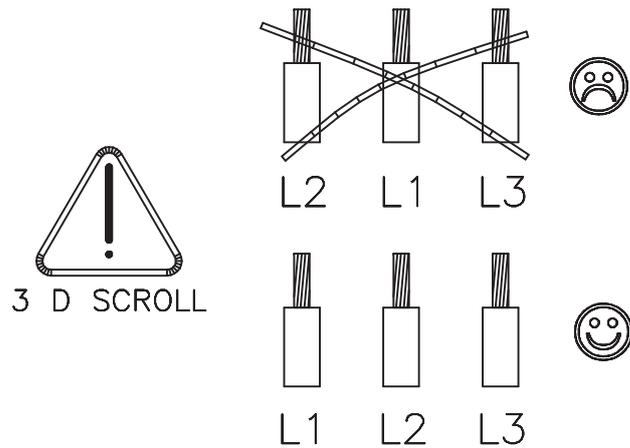
**Note:** Check phase rotation prior to start compressor and make sure phase order is correct. Failure to do so may result on compressor damage.
