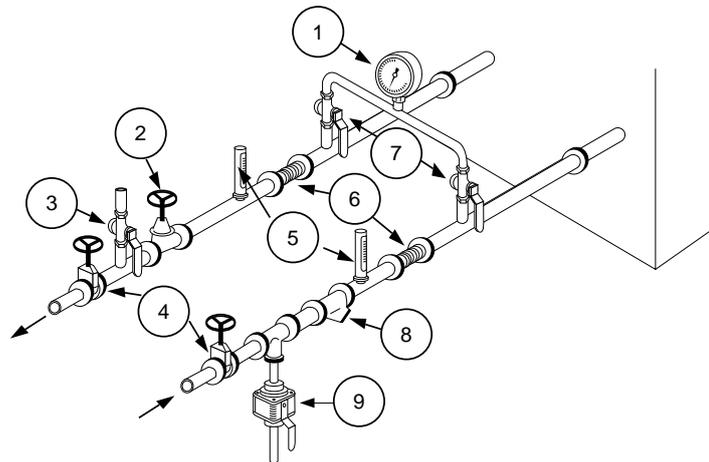
1 = Pressure gauges: show entering and leaving water pressure
