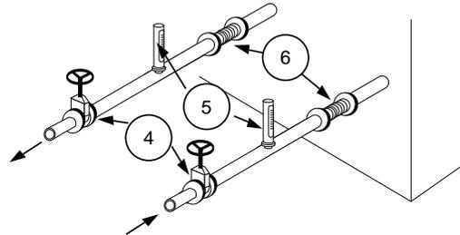
*Figure 2 - Connection of units without hydraulic module - Evaporator and condenser sides*
