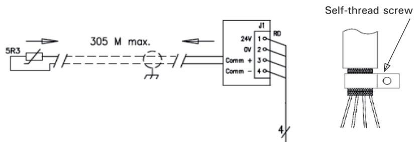
**Figure 11 - CGWN and CCUN main power supply connection (205-211)**
