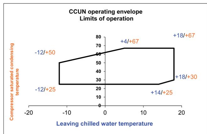
**Note:** CGWN 205 to 211 have a maximum condenser leaving water temperature of 60°C.
