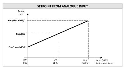
Correction calculation with ratiometric input (b20=1):
