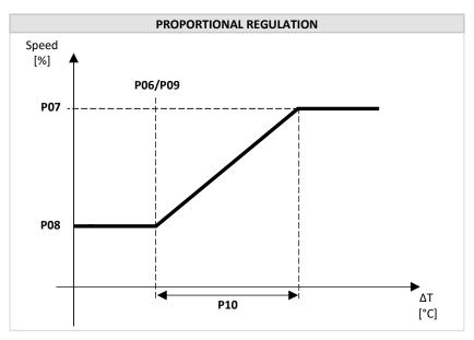
In practice, in cooling mode, if the temperature difference between the inlet and outlet is greater than PO9 + P10, the circulator runs at maximum speed, but if the difference is less than PO9 - 0.2°C, it runs at minimum speed; in the remaining cases, the pump modulates the speed proportionally. In heating mode, the same considerations apply, replacing parameter P06 with parameter P09. In sanitary production the circulator always runs at maximum speed.
