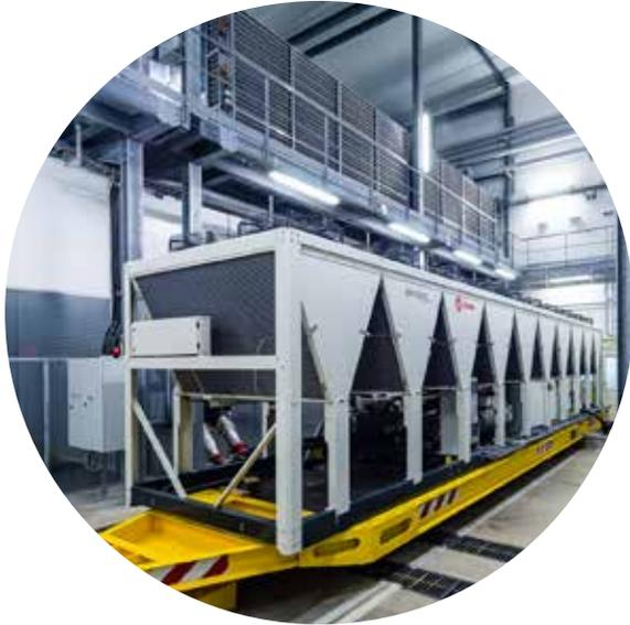
Sintesis unit RTAF 310T under test
