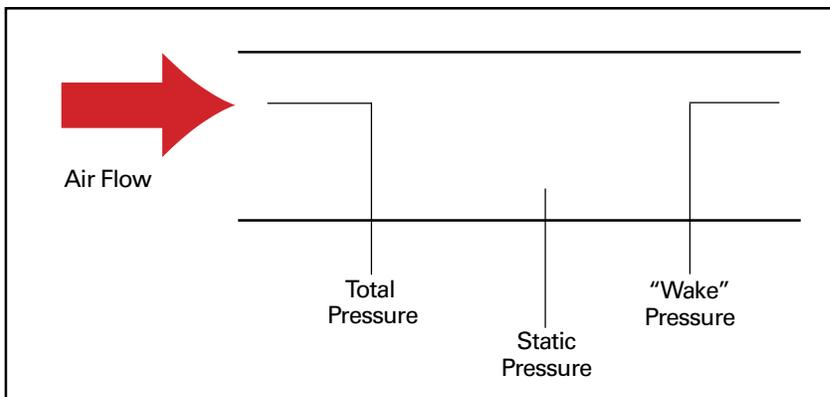
The velocity pressure is defined as the difference between the total pressure in the duct and the static pressure in the duct:
