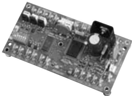
**Direct digital control (DDC) systems** became available as advances in computer technology made small microprocessors available and affordable. Much of the hardware in DDC systems is similar to analog electronic systems. The primary difference is that DDC controllers allow system integration, remote monitoring, and adjustment. The microprocessor is programmed using software that gives the controller a higher level of capability than either the pneumatic or analog electronic options.
