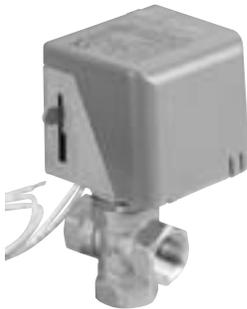
The most important factor when sizing valves is the coefficient of velocity or  $C_v$ . The  $C_v$  is defined as the flow rate, in gallons of 60°F (15.56°C) water, that will pass through the valve in one minute with a one pound pressure drop. The coefficient of velocity, which is commonly called the flow coefficient, is an industry standard rating. Valves having the same flow coefficient rating, regardless of manufacturer, will have the same waterside performance characteristics.
