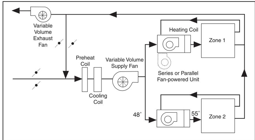
Airside savings are obtained using a combination of lower air temperature and intelligent control strategies. The ability of the VAV unit to communicate information is vital to system coordination.
