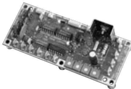
**Analog electronic control systems** began to be used in the 1970s and 1980s. Cost effective and reliable transistors, resistors, relays, and triacs (electronic relays) allowed analog electronics to become a substitute for pneumatic controls. Analog electronic controls use varying voltage signals to change an output in response to a monitored variable.
