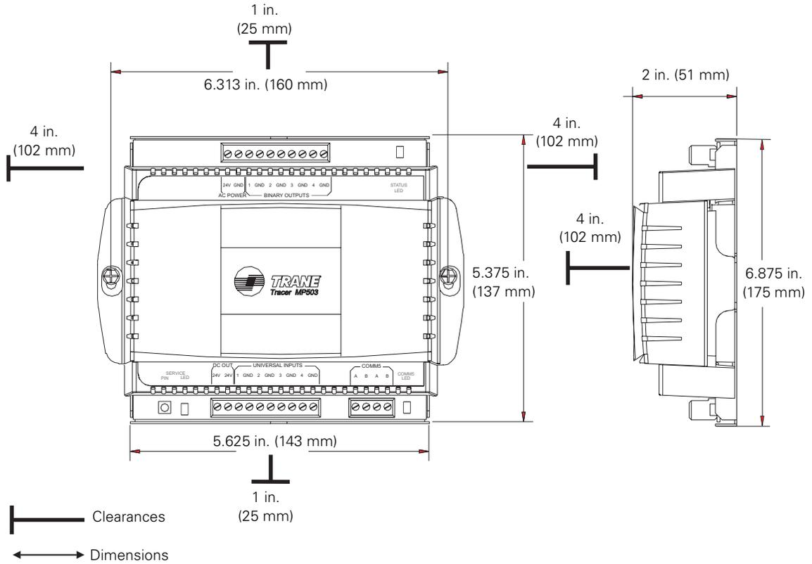
**Figure 2. Dimensions and clearances for the metal-enclosure version I/O module**
