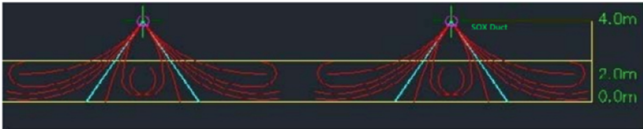
Airflow Distribution of DurkeeSox Air Dispersion System
