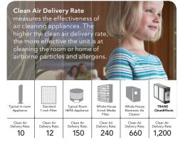
Clean air delivery rate (efficiency times airflow rate) is recognized by the Federal Trade Commission (FTC) and the Environmental Protection Agency (EPA) as a fair and objective measure of various air cleaner technologies. Ratings reflect cubic feet per minute of clean air delivered for a typical 3-ton heating and cooling system: the higher the value, the more effective the air cleaner.
